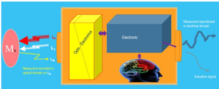
**Figure 3:** Illustration of the optoelectronic unit of a photonic sensor. It is in charge of producing and controlling the photonic beams or Light (if required) to carry out the object’s interrogation or/and pumping tasks. It is also in charge of achieving the photodetection, and all required additional processes, to
