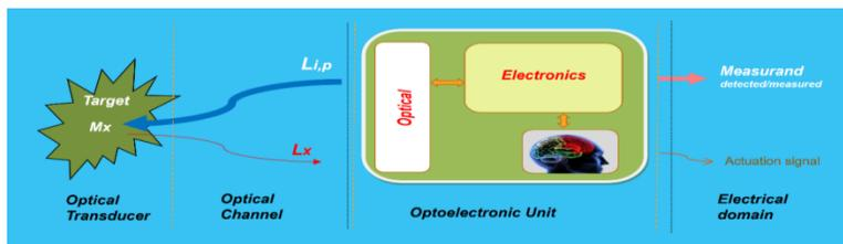
**Figure 4:** Illustration of the photonic sensor concept and its block diagram. The photonic sensor provides representative and faithful electrical signals of the measurands on/in a given object or target. When a PS is equipped with intelligence and provides actuation signals, it is transformed into a Smart
