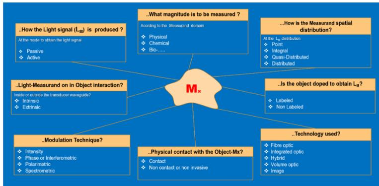
**Figure 5:** Types of photonic sensors taking into consideration aspects concerning the measurand (M<sub>x</sub>) on/in the object (O<sub>y</sub>) and the modulated Light (L<sub>M</sub>). Courtesy of the author.
