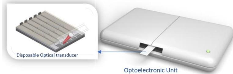
**Figure 11:** Illustration of the optoelectronic unit and a very ample view of the disposable optical bimodal waveguide (BiMW) interferometric technology considered in the CONVAT project. Made by the author based on material courtesy of Laura Lechuga [64].
