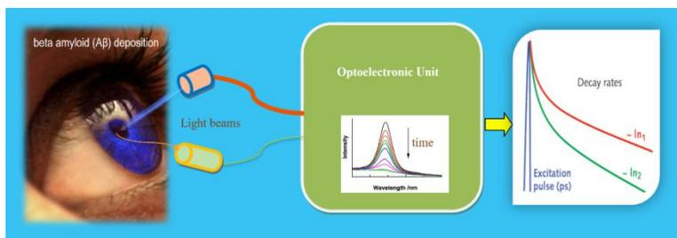
**Figure 17:** Illustration of a BioPhotonic Sensor (BioPS-FLES) for early detection of Alzheimer's disease. The excitation laser pulsed light from the optoelectronic unit in the interaction with the lens of the eye provokes a fluorescent light (LM) that, after detection and adequate treatment in the OU, the output is given based on the decay times. The higher the beta-amyloid, the lower the fluorescent decay times [105]. Courtesy of the author.
