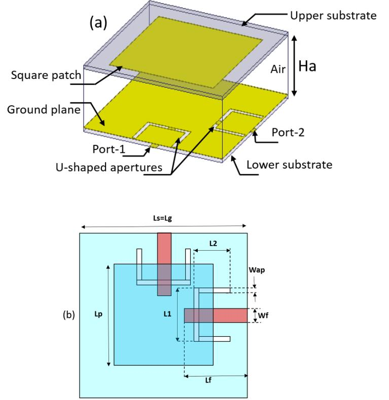
Fig. 2. Structure of the proposed dual-polarized aperture coupling antenna: (a) 3D view, (b) Top view.
