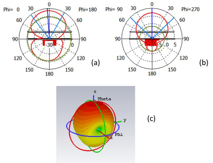
Fig. 7. Diagram pattern: (a) E-plane and (b) H-plane. (c) 3D diagram pattern.
