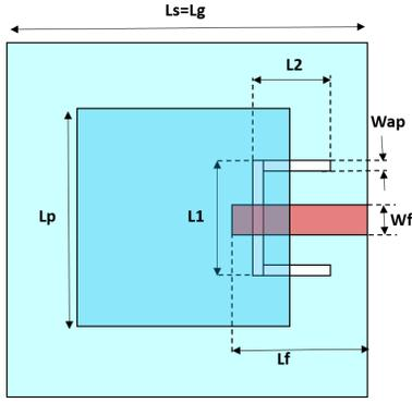
Fig. 1. Top view of the antenna with single feed line.
