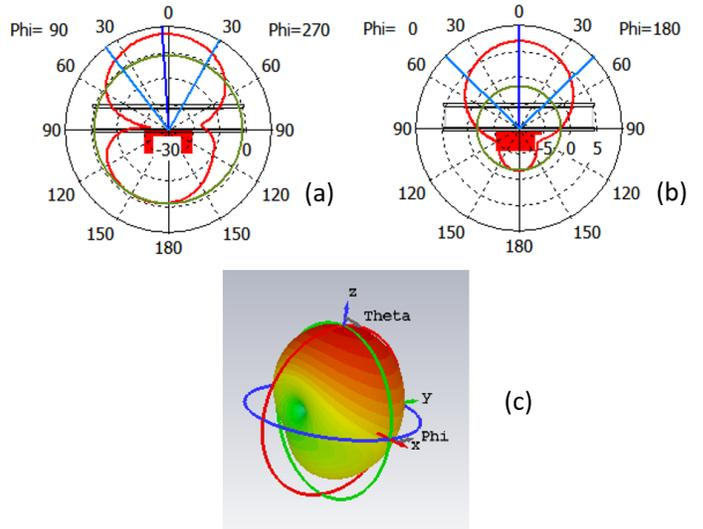
Fig. 8. Diagram pattern: (a) E-plane and (b) H-plane. (c) 3D diagram pattern.
