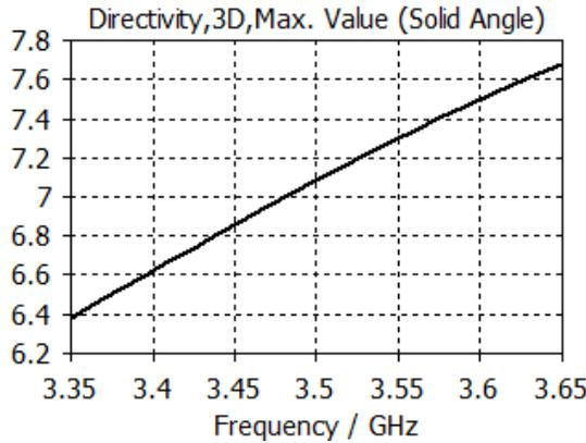
Fig. 5. Directivity of the proposed antenna.
