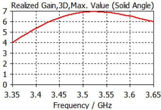
Fig. 4. The gain of the proposed antenna.
