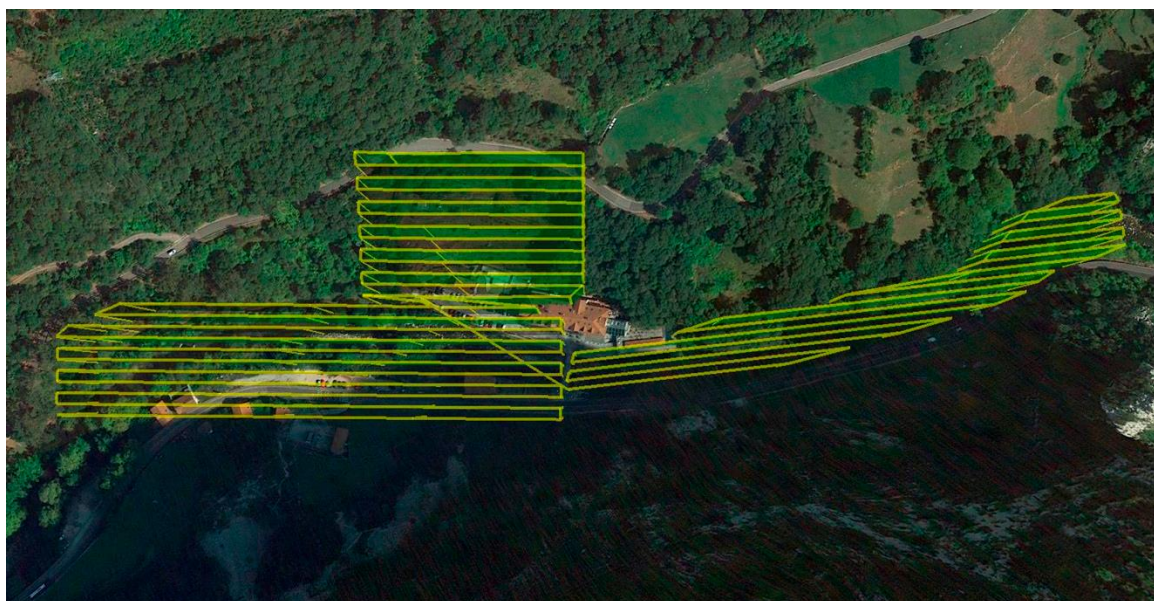
Figure 3. Flight geometry on simple grid configuration performed over the riverbed and spa facilities.
