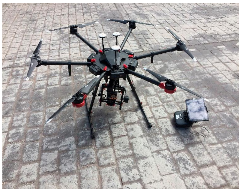
Figure 2. UAV DJI Matrice 600 and WIRIS Pro dual sensor used for image capture.
