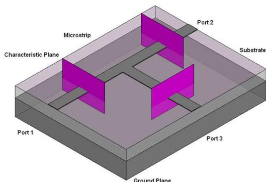
Figure 3: Characteristics planes of microstrip tee junction.
