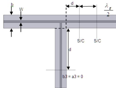
Figure 11: Definition of characteristic planes of right angled finline tee-Junction.
