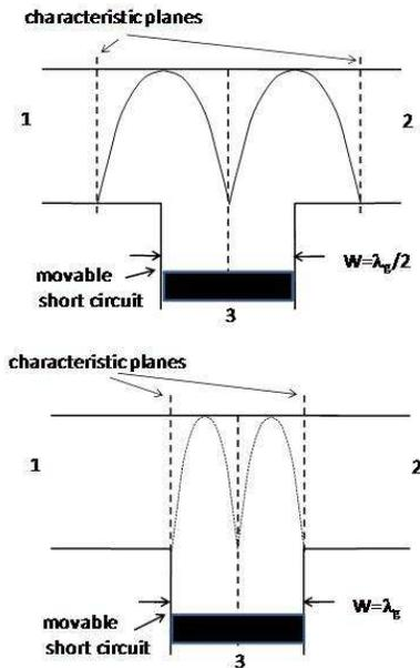
Figure 5: Characteristics planes at two different frequencies.
