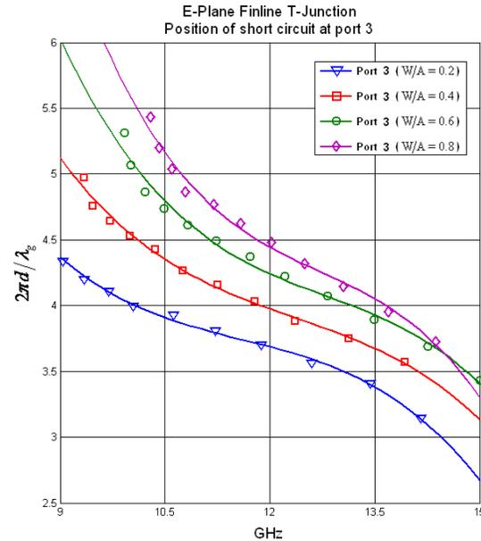
Figure 13: Calculated characteristic planes of the  $E$ -plane unilateral finline tee-junction at port 3 between the frequency range of 9 to 15 GHz.
