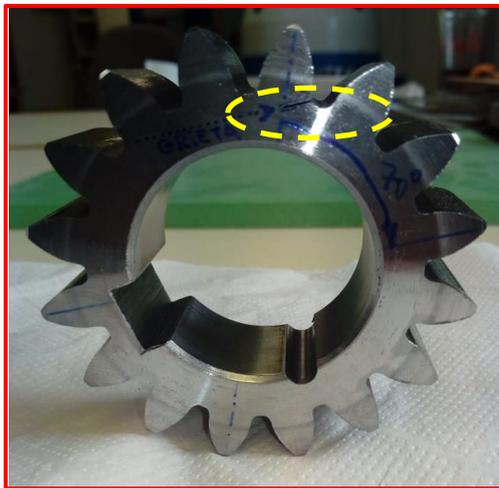
**Fig. 4.** Crack on the test sun gear
