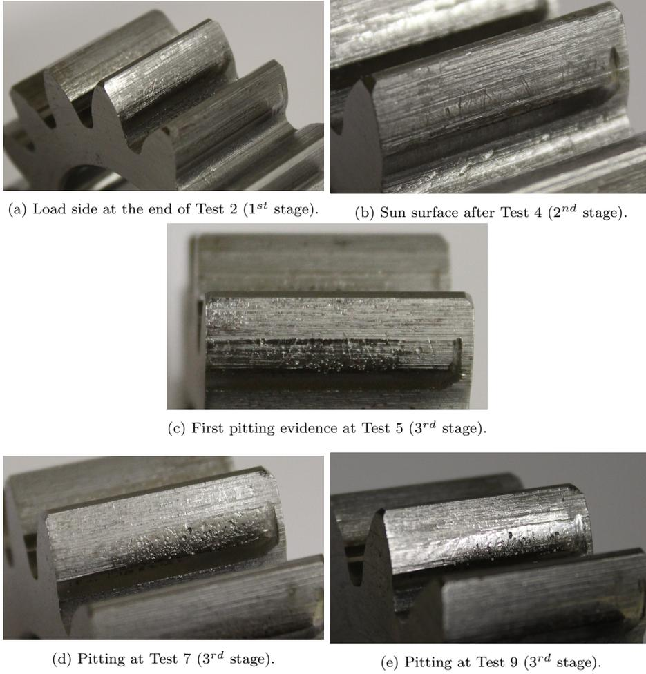
Figure 10: Sun gear active surfaces photographed during the inspections at the end of the tests.
