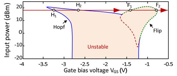
Fig. 1. Bifurcation loci of a test-bench power amplifier.
