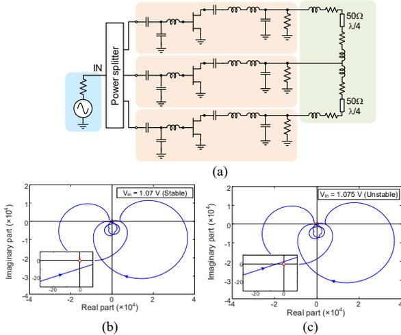
Fig. 2. Test-bench of three power amplifiers under output coupling effects. The Nyquist criterion is applied to the characteristic determinant for two input-amplitude values. (a) Stable. (b) Unstable.
