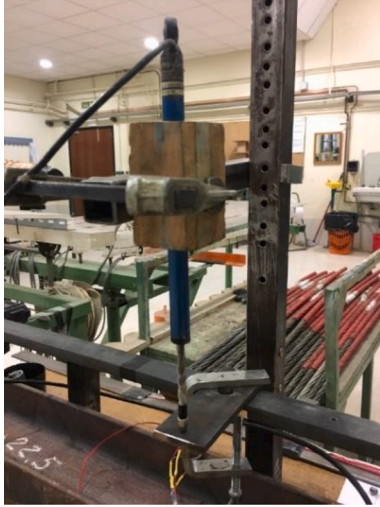
Fig. 5. Potentiometer displacement transducer unit (Penny Giles, SLS095 model).
