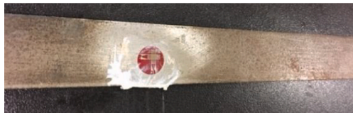
Fig. 4. Bidirectional strain-gauge model Tokyo Sokki FCA-3-11-1L.
