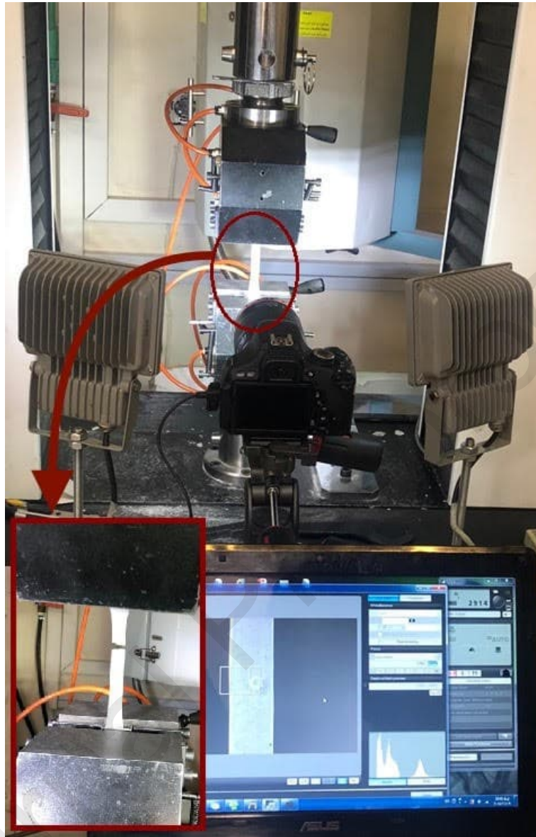
Fig. 5. Un-notched specimen inside the tensile testing machine and the DIC method.
