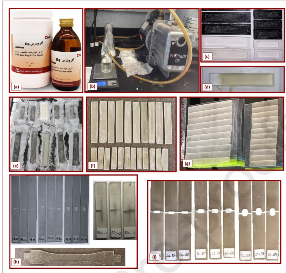
Fig. 2. Preparing the dental material and the test samples: (a) the dental material components (b) the vacuum pump machine (c) the molds made by the 3D printing method (d) the sample not separated from the mold (e) use of the Dacron fabrics (f) the samples after separating from the molds (g) after sizing the samples (h) after machining to create the desired notches (i) the broken samples and the fracture paths.
