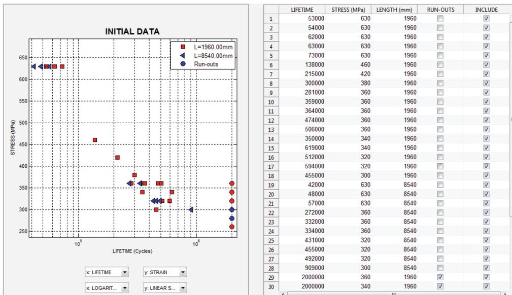
Fig. 1: Input data for S-N fatigue analysis for prestressing wires with two different lengths
