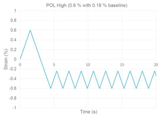
Fig. 3. Variable amplitude fatigue test.
