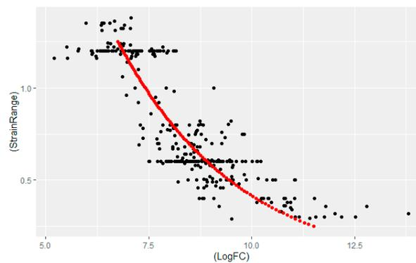
Fig. 1. Selection of fatigue test data in a PWR environment (in red, theoretical model).
