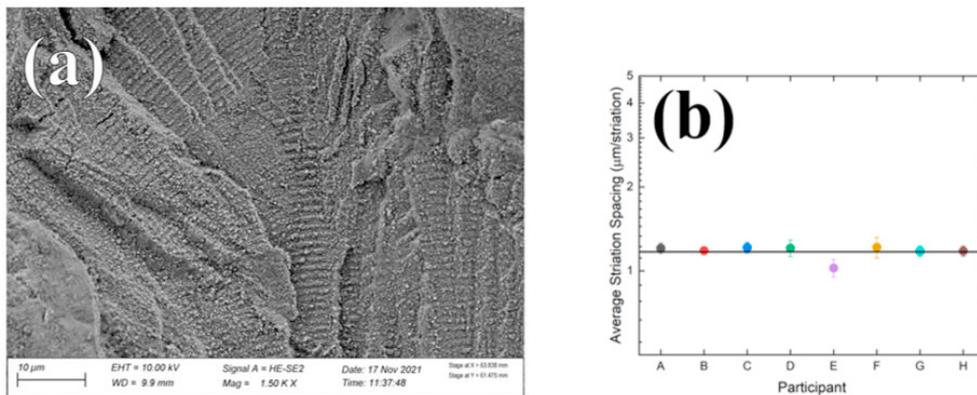
Fig. 4. SEM image of fatigue fracture surface. a) Analyzed area with fatigue striations; b) Measurements by different laboratories.
