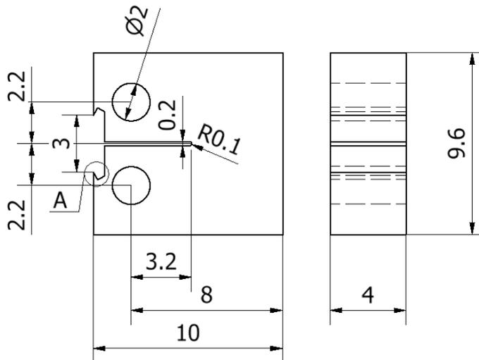
Figure 2. Test specimen dimensions (mini CT), as proposed for the project.
