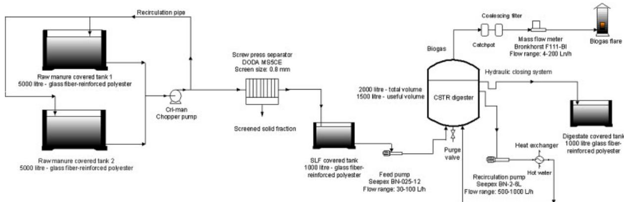
Figure 1. Scheme of the pilot installation.
