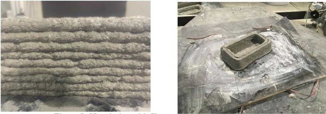
302 **Figure 5: 3D printing with fibers**
