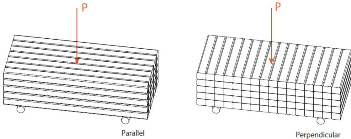
326 **Figure 6:** Flexural strength test directions. Left parallel and right perpendicular
