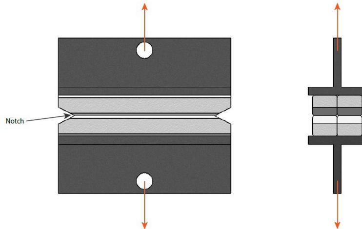
*Figure 8: Interlayer bond strength test*
