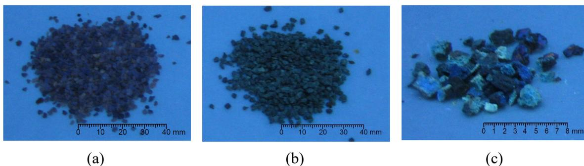
276 Figure 12. (a) Empty capsules (b) filled with rejuvenator (c) broken sepiolite under UV light
