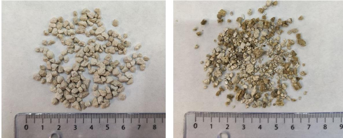
158 Figure 2. Detail of porous aggregates: sepiolite (left); vermiculite (right)
