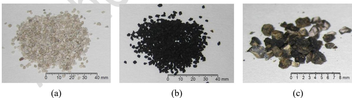
274 Figure 11. (a) Empty capsules (b) filled with rejuvenator (c) broken sepiolite under visible
