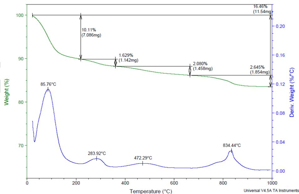
Figure 5. Thermogravimetric curve of sepiolite
