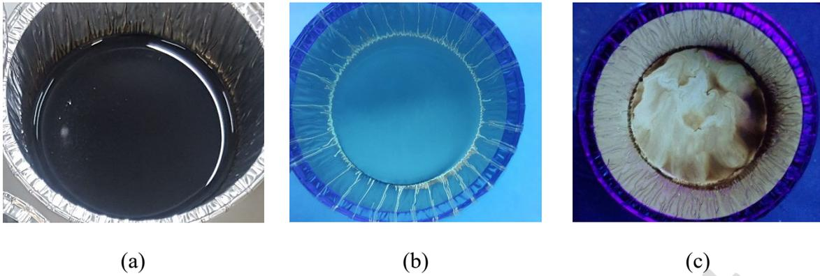
142 Figure 1. (a) Rejuvenator sample under visible light, (b) under UV light and (c) bitumen
