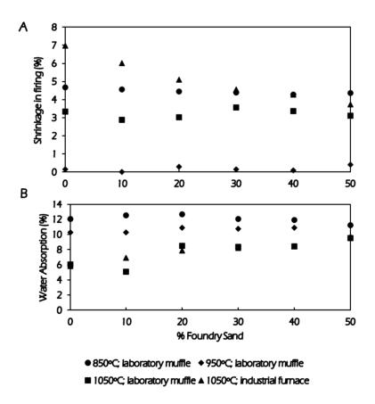
Figure 2.26. Technological characterisation of the clay-sand pieces: a) shrinkage firing and b) water absorption.
