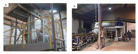
Figure 2.29. Company equipment: A) Laminator; B) Extruder.
