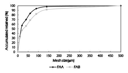
Figure 2.3. Particle size distribution of Coal Fly Ash A and B.
