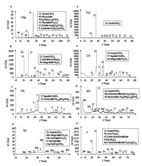
Figure 2.17. XRD of raw material and FBs: (A) Clay; (B) FS (Foundry Sand-cast iron); (C) FSL (Foundry Sludge); (D) SD (Steel Dust); (E) FS2 (Foundry Sand-ductile iron); (F) CA (Cupola Bottom Ash); (G) WS (Wet Sands); and (H) F (Fines).
