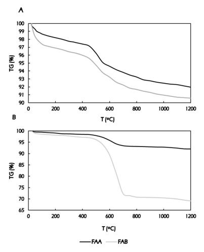
Figure 2.5. Thermogravimetric behaviour of A) Clay A and Clay B; B) FAA and FAB.
