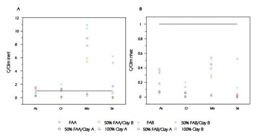
Figure 2.7. The concentration of contaminants of FA/Clay bricks regarding the inert waste landfill limits (A) and the non-hazardous waste landfill limits (B) according to Decision 2003/33/EC.
