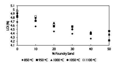
Figure 2.25. Influence of temperature on weight loss (LOI) of FS/clay mixtures.
