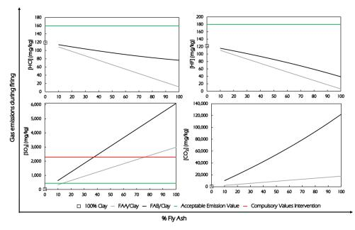
Figure 2.13. Estimation of HCl, HF, SO<sub>2</sub>, and CO<sub>2</sub> emissions for mixtures performed with FAA/Clay B and FAB/Clay B during the firing process, including reference emission values proposed by I. Gonzalez et al. (González et al., 2011).
