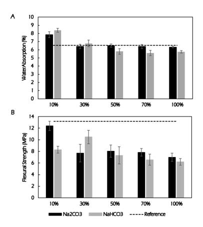
Figure 3.11. Influence of the use of Na<sub>2</sub>CO<sub>3</sub> Powder and HNaCO<sub>3</sub> Powder on the technological properties: (a) Water absorption; (b) Flexural Strength.
