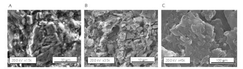
Figure 2.12. Microstructure FESEM images taken at different regions of 100% Clay B.
