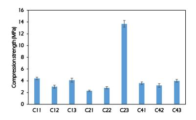
Figure 4.11. Compressive strength results (14 days) of alkali activated binders.
