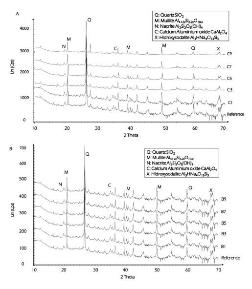
Figure 3.13. a) XRD of carbonate-based geopolymer; b) DRX of bicarbonate-based geopolymer.
