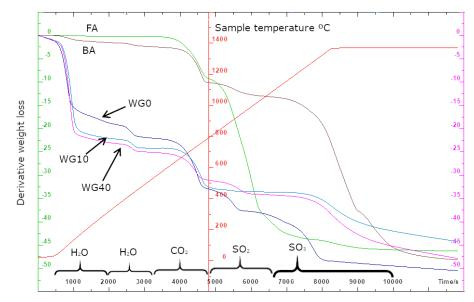
Figure 4.20. TG-DTG Fly Ash (FA), Bottom Ash (BA), WG0, WG10 and WG40 binders.
