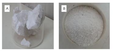
Figure 3.3. CaO rocks before (A), and after crushing (B).
