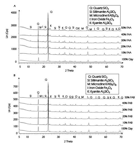
Figure 2.8. XRD patterns of: (A) FAA/Clay fired bricks; (B) FAB/Clay fired bricks.
