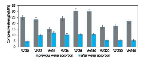
Figure 4.18. Compressive strength before and after the water absorption of WG binders (Table 4.10 Mix Design).
