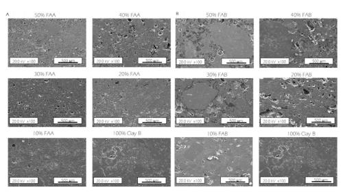
Figure 2.9. FESEM images of fired clay bricks: (A) FAA/Clay fired bricks; (B) FAB/Clay fired bricks.
