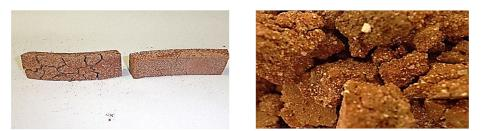
Figure 4.5. Alkali activation feasibility results: (A) Overall bricks view (left picture); .(B) Zoomed bricks view (right picture).
