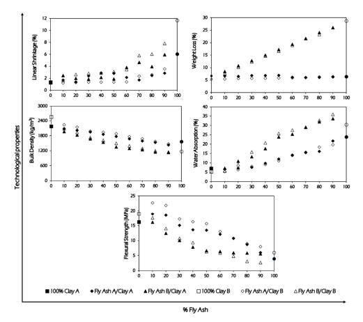
Figure 2.6. Main technological properties of fired clay bricks.
