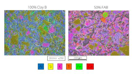
Figure 2.11. FESEM images and mapping of elements of samples 100 % Clay B and 50 % FAB/Clay B.
