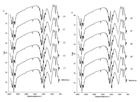
Figure 3.14. FTIR a) Carbonate-based geopolymer; b) Bicarbonate-based geopolymer.
