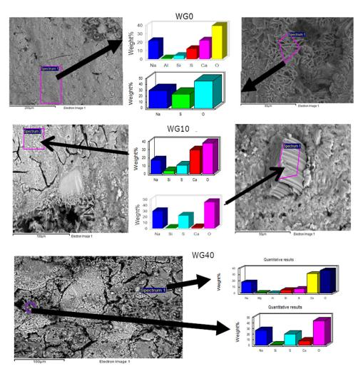
Figure 4.21. SEM-EDX WG0, WG10, and WG40 binders.
