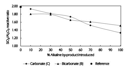
Figure 3.12. SiO<sub>2</sub>/Al<sub>2</sub>O<sub>3</sub> reactive ratio of the alkali-activated materials.
