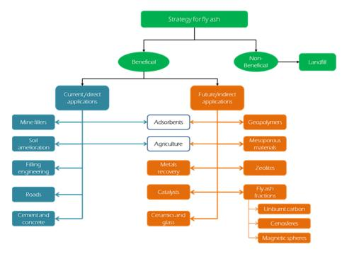
Figure 2.1. Scheme of the different applications of Coal Fly Ashes.
