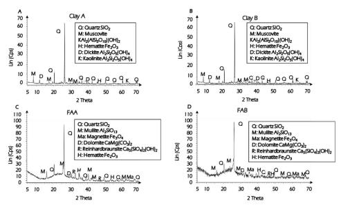
Figure 2.4. XRD pattern of Clay A (A), Clay B (B), FAA (C), and FAB (D).
