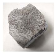
Figure 4.12. No clay alkali activate material.
