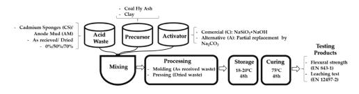
Figure 3.16. The methodology applied for the geopolymeric formulations development.
