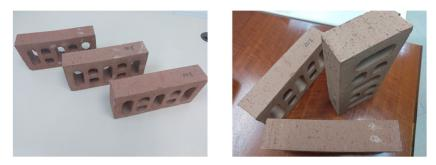
Figure 2.31. The visual appearance of the FS-Clay bricks.
