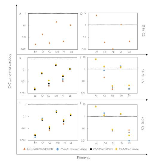
Figure 3.20. Contaminant concentration of geopolymers using commercial (C) or alternative (A) activator incorporating Cadmium Sponge (CS) with/without pretreatment regarding the non-hazardous waste landfill disposal limits: Ba, Cr, Cu, Mo, Ni, and Sb with 0 %, 50 % and 70 % (CS), (A), (B) and (C) respectively; As, Cd, Pb, Se, and Zn with 0 %, 50 %, and 70 % Cadmium Sponge (CS), (D), (E) and (F), respectively.
