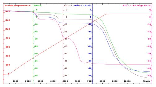
Figure 4.1. Bottom CFBC ashes.TG-DTG. A0: particle size<0.3mm; A3: 0.3mm<size particle<0.6 mm; A6: particle size<0.6 mm. and A: raw ashes.
