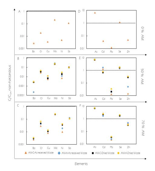
Figure 3.21. Contaminant concentration of geopolymers using commercial (C) or alternative (A) activator incorporating Anode Mud (AM) with/without pre-treatment regarding the nonhazardous waste landfill disposal limits: Ba, Cr, Cu, Mo, Ni, and Sb with 0%, 50%, and 70% Anode Mud (AM); (A); (B) and (C) respectively; As, Cd, Pb, Se, and Zn with 0%, 50% and 70%, Anode Mud (AM); (D); (E) and (F), respectively.
