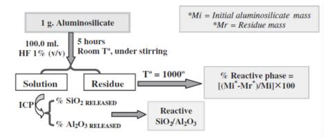
Figure 3.9. An experimental procedure was followed to quantify the percentage in weight of the potentially reactive phase and the reactive  $SiO_2/Al_2O_3$  ratio in the starting aluminosilicates (Ruiz-Santaquiteria et al., 2013).
