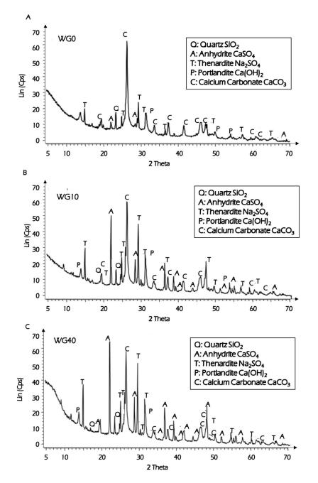
Figure 4.19. XRD patterns of reaction products after 28 days: (A) WG0 binder; (B) WG10 binder; (C) WG40 binder.
