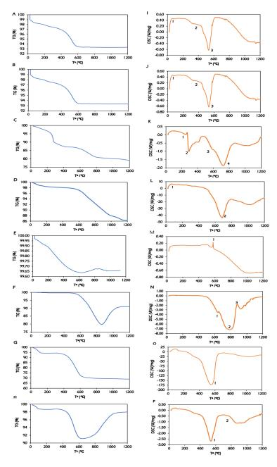
Figure 2.18. Thermal characterisation of raw materials and Foundry by-products. On the left: Thermogravimetric analysis (TGA); Right: Differential Scanning Calorimetry (DSC): (A) and (I) Clay; (B) and (J) FS (Foundry Sand-cast iron); (C) and (K) FSL (Foundry Sludge); (D) and (L) SD (Steel Dust); (E) and (M) FS2 (Foundry Sand-ductile iron); (F) and (N) CA (Cupola Bottom Ash); (G) and (O) WS (Wet Sands); and (H) and (P) F (Fines).
