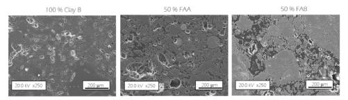
Figure 2.10. FESEM images of 100 % Clay B and 50 % FAA and FAB/Clay B fired clay bricks.
