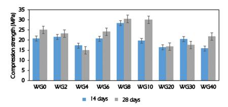
Figure 4.16. Compressive strength of WG binders (Table 4.10) after 14 and 28 days.
