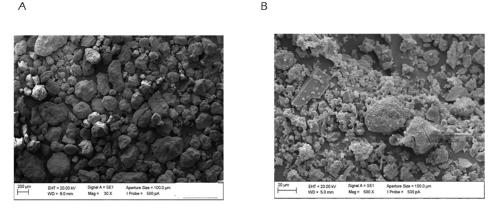
Figure 4.15. SEM micrographs of CFBC ashes: (A) Fly Ash; (B) Bottom Ash.
