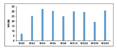
Figure 4.17. Water absorption of WG binders (Table 4.10 Mix Design).
