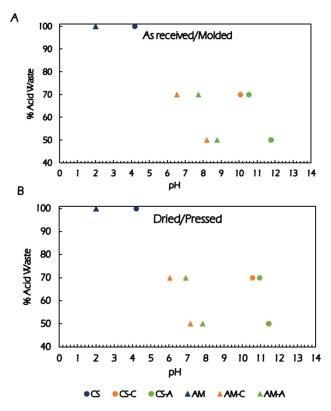
Figure 3.17. pH values of leachates of acid waste Cadmium Sponge (CS) and Anode Mud (AM) S/S: (A) as-received waste, processed by moulding; (B) pretreated waste, processed by pressing.
