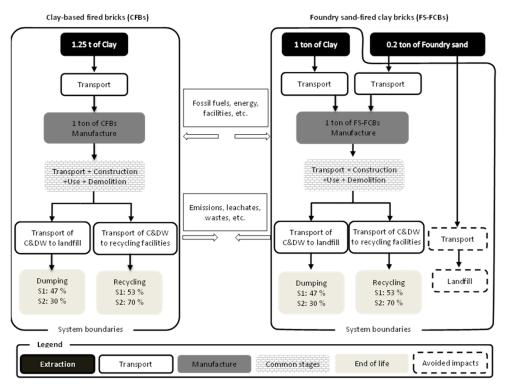
Figure 2.32. Life cycle flow diagram of the bricks produced (B and B + S) to apply the LCA tool.
