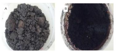
Figure 3.15. Acid waste used in this work: (a) Cadmium Sponges (CS); (b) Anode Mud (AM).
