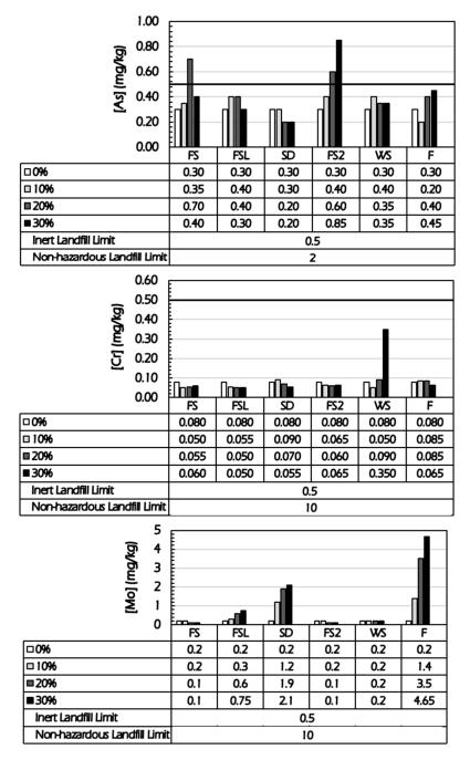
Figure 2.23. Average concentrations of As, Cr, and Mo in mg/kg in the FB-FCBs (Foundry byproducts-fired clay bricks). FS (Foundry Sand-cast iron); FSL (Foundry Sludge); SD (Steel Dust); FS2 (Foundy Sand-ductile iron); CA (Cupola Bottom Ash); WS (Wet Sands); and F (Fines).
