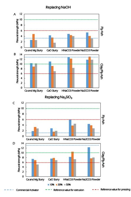
Figure 3.7. Influence of the utilisation of alkaline by-products on the flexural strength by substituting NaOH using as aluminosilicate source: (a) Fly Ash; (b) Fly Ash/Clay, and by substituting Na<sub>2</sub>SiO<sub>3</sub> using as aluminosilicate source: (c) Fly Ash; (d) Fly Ash/Clay.
