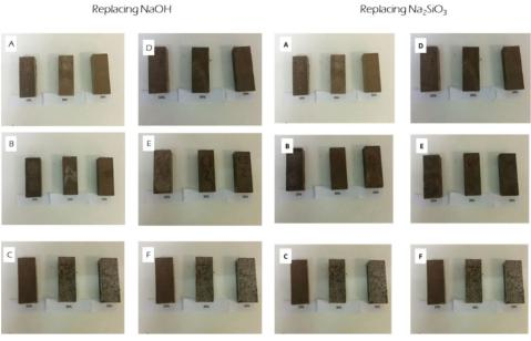
Figure 3.5. Geopolymers formation with NaOH/Na<sub>2</sub>SiO<sub>3</sub> substitution of the following alkaline by-products: Ca and Mg Slurry (A), HNaCO<sub>3</sub> Powder (B), Ca-Si-CaCO<sub>3</sub>(OH)<sub>2</sub> Sludge (C), CaO Slurry (D), Na<sub>2</sub>CO<sub>3</sub> Powder (E), CaO Rocks (F).
