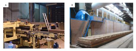
Figure 2.30. Cutting and firing of the pieces: A) Cutter; B) Tunnel kiln.
