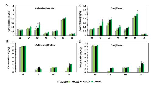
Figure 3.19. Mobility of contaminants of Anode Mud (AM) S/S – commercial (C)I/alternative (A) activator: (A) and (B) As-received waste and moulded; (C) and (D) Dried waste and pressed.
