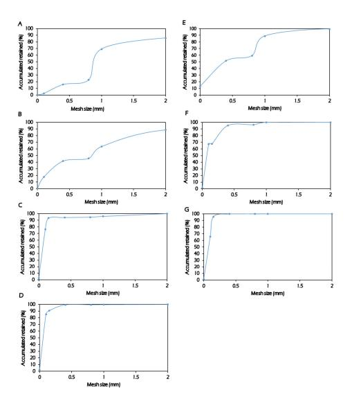
Figure 2.16. Particle size distribution of FBs: (A) FS (Foundry Sand-cast iron); (B) FSL (Foundry Sludge); (C) SD (Steel Dust); (D) FS2 (Foundry Sand-ductile iron); (E) CA (Cupola Bottom Ash); (F) WS (Wet Sands); and (G) F (Fines).
