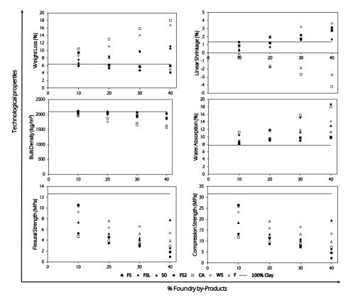
Figure 2.20. Technological properties of foundry by-products-fired clay bricks (FB-FCBs). FS (Foundry Sand-cast iron); FSL (Foundry Sludge); SD (Steel Dust); FS2 (Foundy Sand-ductile iron); CA (Cupola Bottom Ash); WS (Wet Sands); and F (Fines).
