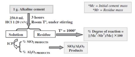
Figure 3.10. The experimental procedure was used to quantify the degree of reaction in the alkaline cement prepared and the  $SiO_2/AI_2O_3$  ratio of the reaction products generated during alkaline activation (Ruiz-Santaquiteria et al., 2013).
