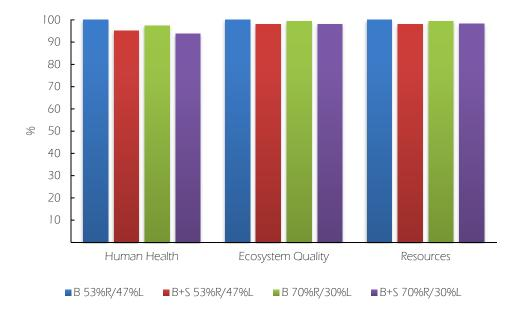
Figure 2.33. Results for each protection area (%), produced by the two types of products, in the two defined management scenarios. Method: Eco-indicator 99 (E) V2.09 / Europe El 99 E / A / Damage assessment / Excluding infrastructure processes.
