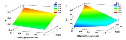
Figure 3.22. Response surface of Cadmium Sponge (CS): pH values and Zn concentration versus waste-geopolymer ratio and NaOH concentration, (A) and (B) respectively.
