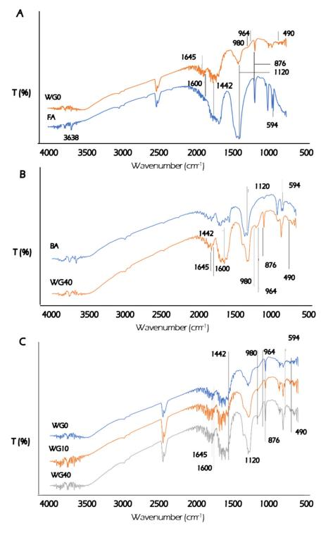
Figure 4.22. FTIR spectra of: (A) Fly Ash and WG0 binder; (B) Bottom Ash and WG40 binder; (C) WG0, WG10, and WG40 binders.
