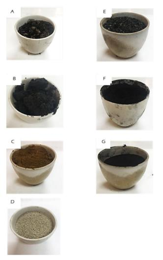
Figure 2.15. Visual appearance of the FBs used: (A) FS (Foundry Sand-cast iron); (B) FSL (Foundry Sludge); (C) SD (Steel Dust); (D) FS2 (Foundry Sand-ductile iron); (E) CA (Cupola Bottom Ash); (F) WS (Wet Sands); and (G) F (Fines).
