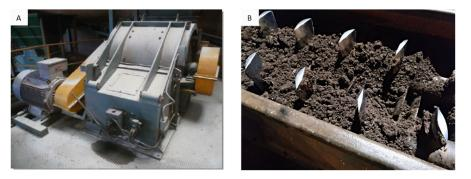
Figure 2.28. Equipment for the conditioning of clay-foundry sand mixtures: A) Hammer mill; B) Kneader.
