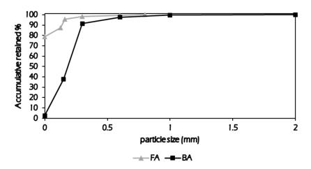
Figure 4.13. Particle size distributions of raw CFBC fly and bottom ashes.
