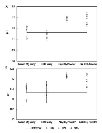
Figure 3.8. Leachate pH values of geopolymers: a) replacing NaOH and b) Na<sub>2</sub>SiO<sub>3</sub> by alkaline by-products.
