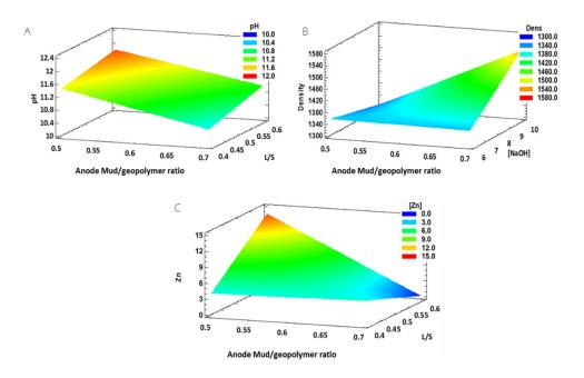
Figure 3.23. Response surface of Anode Mud (AM): pH values (A), geopolymer density (B), and Zn concentration (C) versus waste-geopolymer ratio, liquid-solid ratio, and NaOH concentration.
