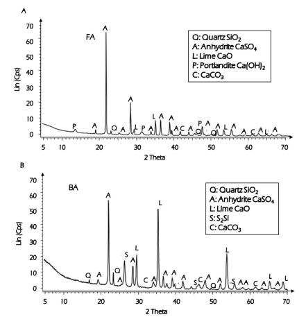
Figure 4.14. XRD patterns of CFCB ashes: (A) fly ash; (B) bottom ash.
