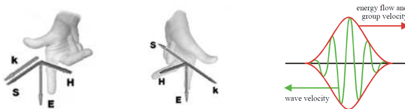
Fig.9. Vectors in right and left handed materials. In left handed materials the Poynting vector has the opposite sign to the wave vector. The anti-parallel phase and group velocities result in backward-wave propagation.
