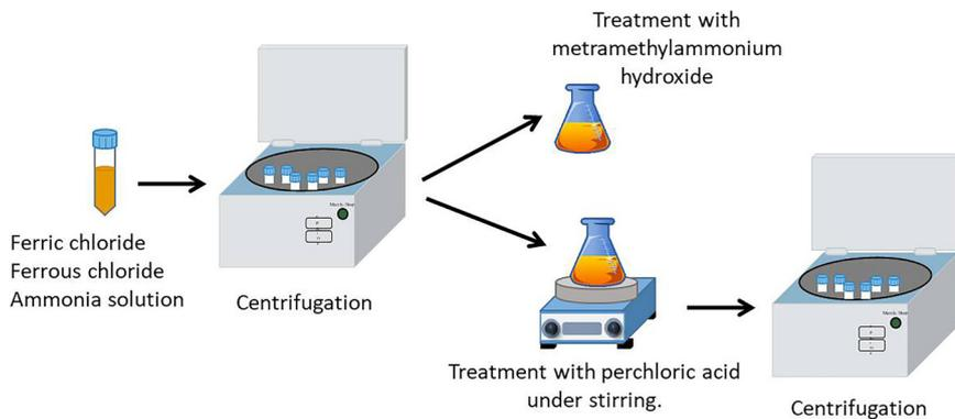
Figure 4: MNPs synthesis based on coprecipitation. Adapted from the study by Massart (1981).
