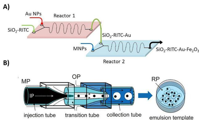
**Figure 12:** Scheme of microreactor systems used to obtain NPs with magnetic coatings.
