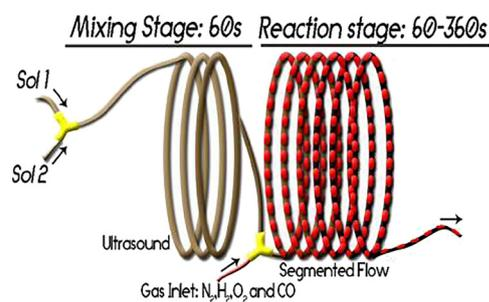
**Figure 7:** Scheme of G/L segmented flow microreactor system employed to synthesize MNPs. Reproduced with permission from Larrea et al. (2015) under the creative common license (<http://creativecommons.org/licenses/by/4.0/>).
