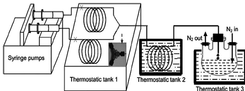
**Figure 9:** Scheme of microreactor system used to perform the simultaneous synthesis and coating of MNPs. Reproduced with changes with permission from Wang et al. (2015).
