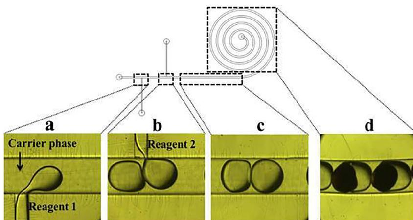
**Figure 8:** Droplet flow microreactor system employed to synthesize MNPs consisting on droplets: (a) dispersion, (b) collision, (c) pairing and (d) fusion. Reproduced with permission from Ma et al. (2019).
