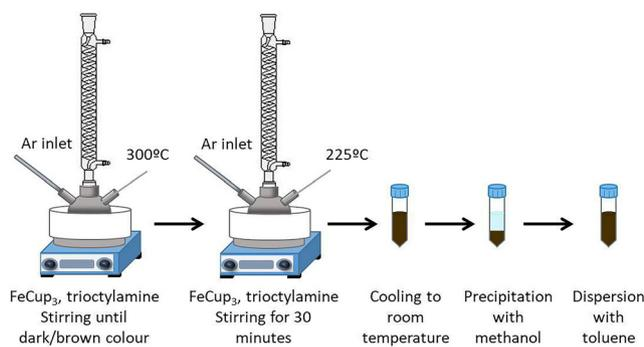
**Figure 5:** MNPS synthesis by the thermal decomposition process. Adapted from Rockenberger et al. (1999).
