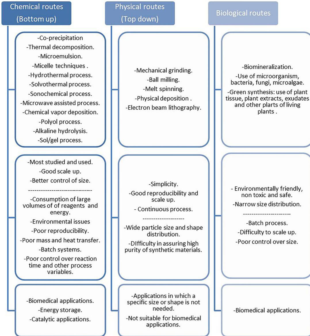
Figure 3: Scheme of technologies to synthesize MNPs, with their advantages, limitations, and potential applications.
