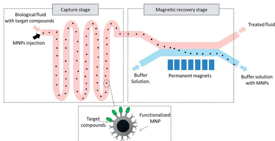
**Figure 1:** Use of MNPs for the capture and micro-magnetoforetic separation of toxins from biofluids.
