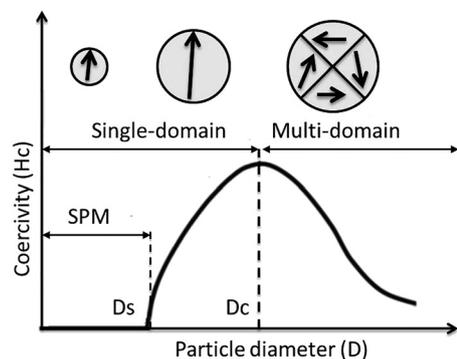
**Figure 2:** Dependence of the coercivity with the particle diameter, for a ferromagnetic material. Adapted from Wu et al. (2016).
