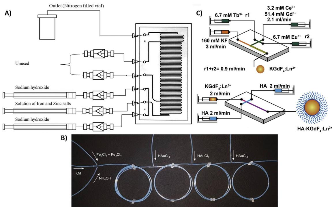
**Figure 10:** Scheme of microreactor systems used to perform the simultaneous synthesis and coating of MNPs.
