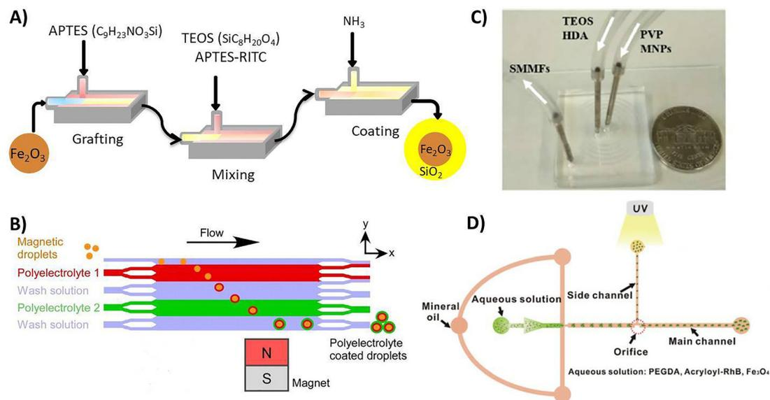
**Figure 11:** Scheme of microreactor systems used to perform the continuous functionalization or coating of MNPs.
