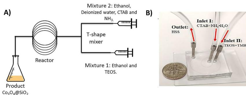
**Figure 13:** Scheme of microreactor systems used to obtain NPs with magnetic coatings. (A) Adapted from Straß et al. (2017) and (B) reproduced with permission from Hao et al. (2019).
