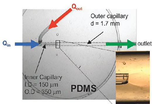
**Figure 6:** Scheme of coaxial flow microreactor systems employed to synthesize MNPs. Reproduced with permission from Abou-Hassan et al. (2008).
