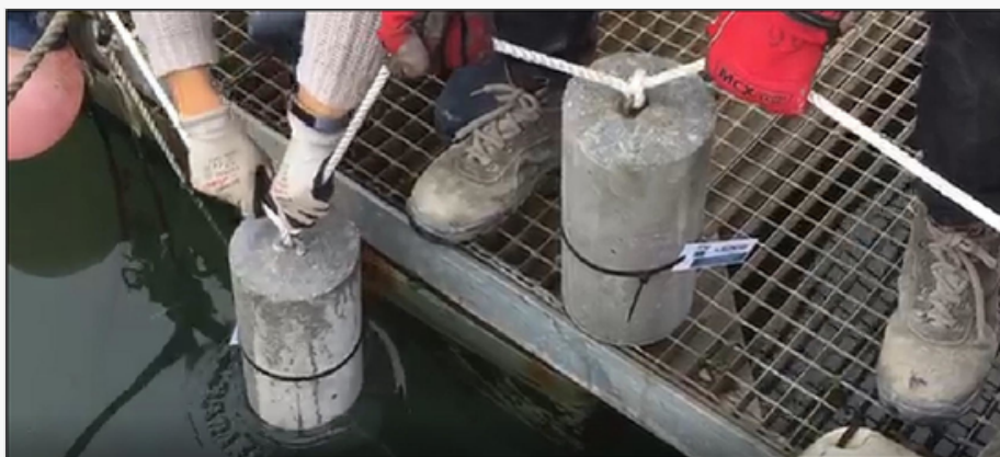
Detail of the specimens and placement in the Santander Bay (Spain).
