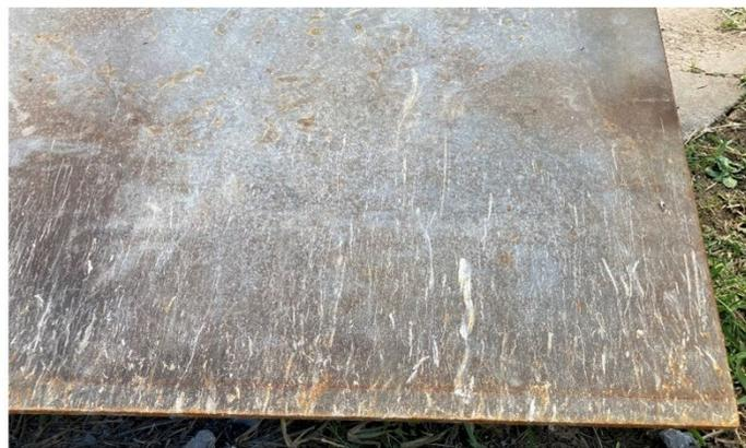
Figure 9. Scratches observed near the tip of the skirts after testing in 1''-3'' gravel.
