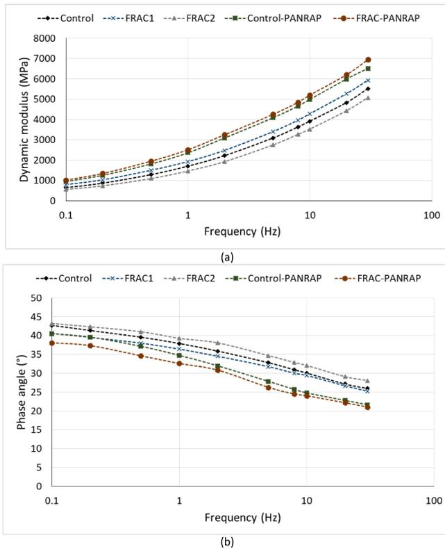
Fig. 8. Stiffness test results; (a) Dynamic Modulus; (b) Phase angle.
