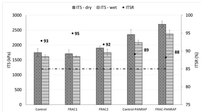
**Fig. 4.** Indirect tensile strength and moisture sensitivity results.
