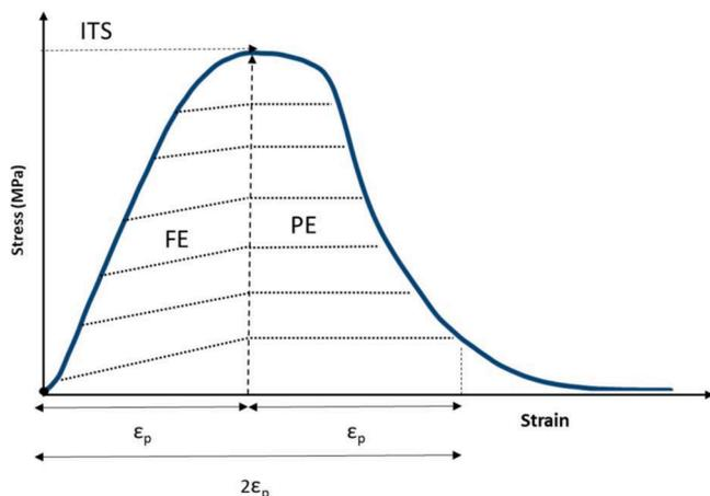
**Fig. 3.** Stress–strain curve recorded from ITS.
