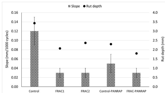
Fig. 6. Slope and Rut depth of wheel tracking test.
