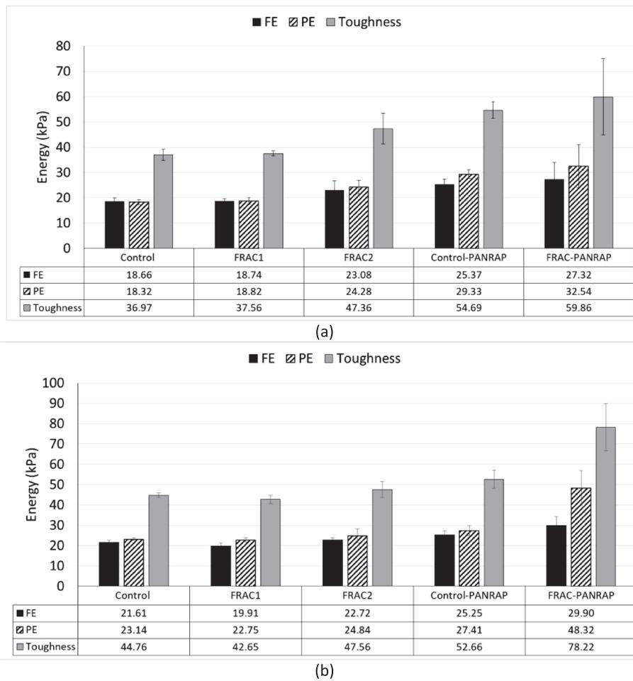
Fig. 5. Fracture properties. Dry conditions (a); Wet conditions (b).
