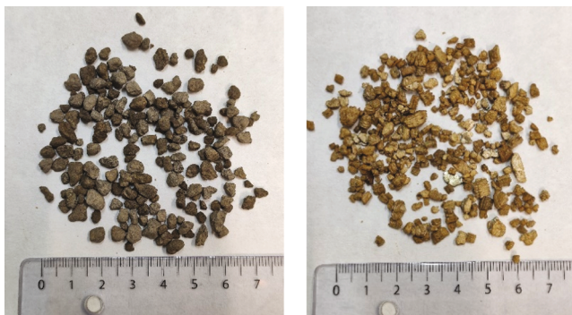
Fig. 2. Sepiolite (left) and vermiculite (right) capsule.
