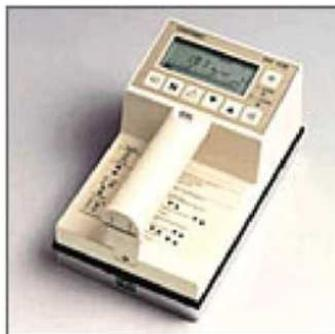
Figura 33: FHT 111 CONTAMAT Contamination Monitor.
