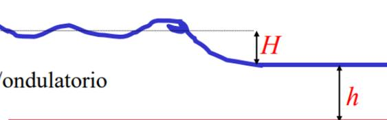
The diagram shows a blue wave profile with a crest that is breaking into a white foam. A vertical double-headed arrow labeled 'H' indicates the wave height, and another labeled 'h' indicates the depth. A red horizontal line is below it.
