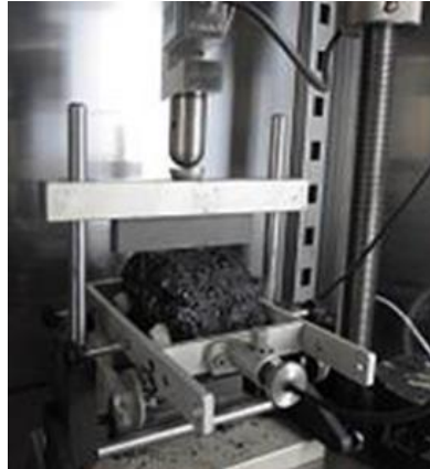
Figure 4. Stiffness test equipment
