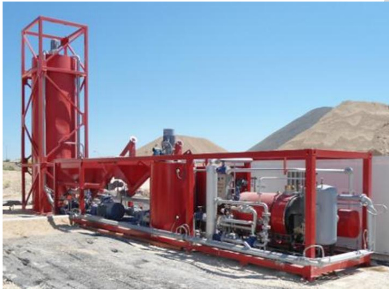
Figure 6. Modification asphalt plant
