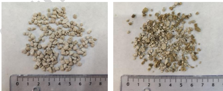
Figure 2. Detail of porous aggregates: sepiolite (left); vermiculite (right)
