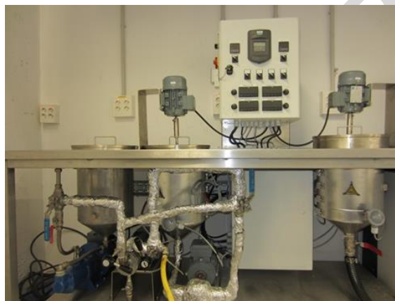
Figure 1. DISPERMAT mixing plant at laboratory level
