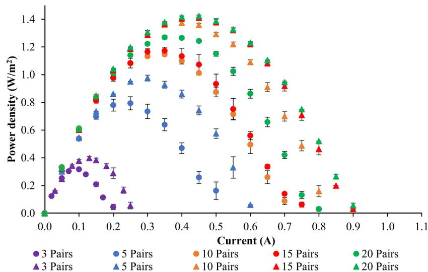
Fig. 2. Spacer thickness influence. Membrane thickness = 30 μm, linear velocity = 2.5 cm·s<sup>-1</sup>. ● = 270 μm spacers. ▲ = 155 μm spacers.
