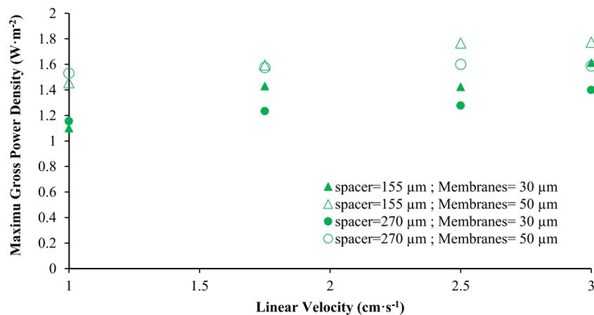
Fig. 6. Linear velocity influence on SGP performance using RED technology. ● = 270  $\mu\text{m}$  spacers and ▲ = 155  $\mu\text{m}$  spacers. ▲ = 30  $\mu\text{m}$  membrane thickness. △ = 50  $\mu\text{m}$  membrane thickness. (For interpretation of the references to colour in this figure legend, the reader is referred to the web version of this article.)
