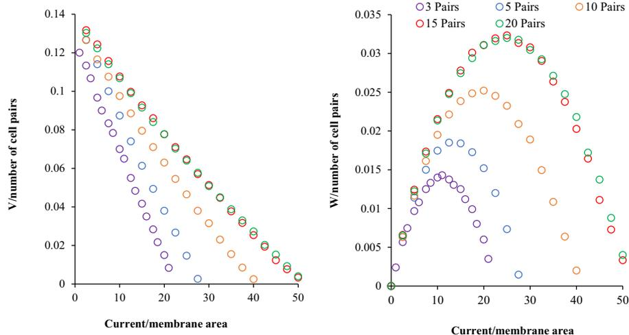
Fig. 4. Polarization and power curves. Membrane thickness = 50  $\mu\text{m}$ , spacer thickness = 270  $\mu\text{m}$  spacers. Linear velocity = 2.5  $\text{cm} \cdot \text{s}^{-1}$ .
