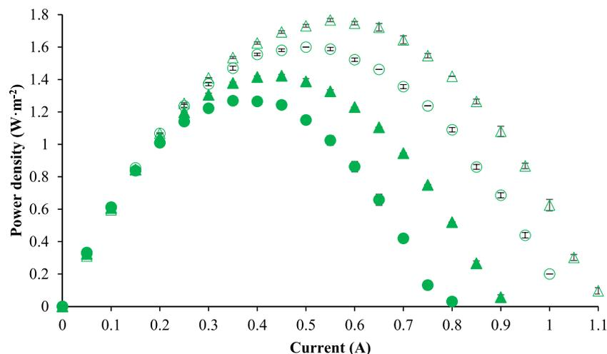
Fig. 3. Membrane thickness influence. Linear velocity = 2.5 cm·s<sup>-1</sup>. ● = 270 μm spacers and ▲ = 155 μm spacers. ▲ = 30 μm membrane thickness. △ = 50 μm membrane thickness.
