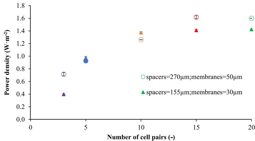
Fig. 5. Membrane pair influence in SGP performance using RED technology when two thickness spacers are employed. Membrane thickness = 50  $\mu\text{m}$ . Linear velocity = 2.5  $\text{cm}\cdot\text{s}^{-1}$ . ○ = 270  $\mu\text{m}$  spacers. ▲ = 155  $\mu\text{m}$  spacers. (For interpretation of the references to colour in this figure legend, the reader is referred to the web version of this article.)
