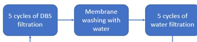
**Figure 7.** Scheme of the automated fouling evaluation assays
