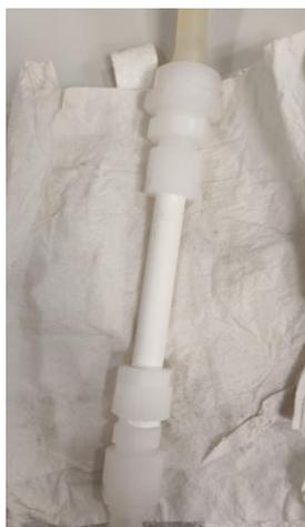
**Figure 4.** *TiO<sub>2</sub> membrane with fittings.*
