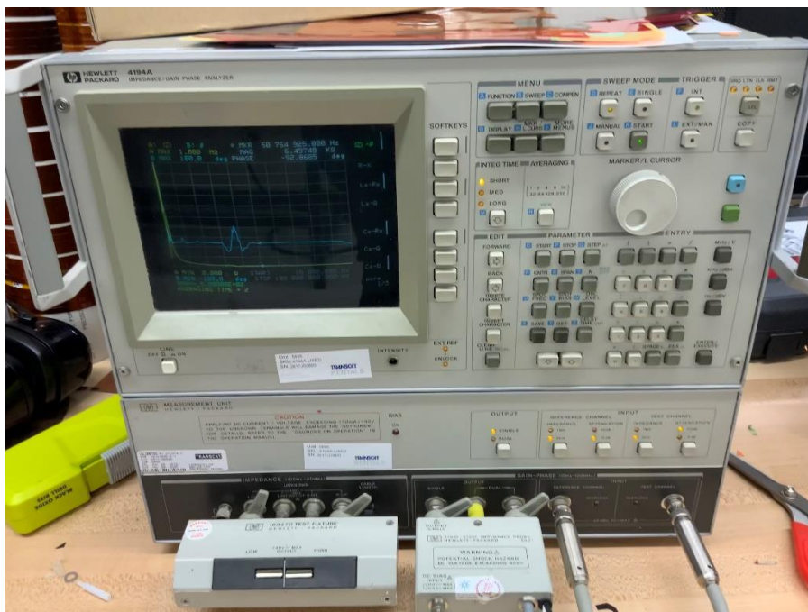
Figure 18. IMPEDANCE/GAIN PHASE ANALYZER (HP – HEWLETT PACKARD)
