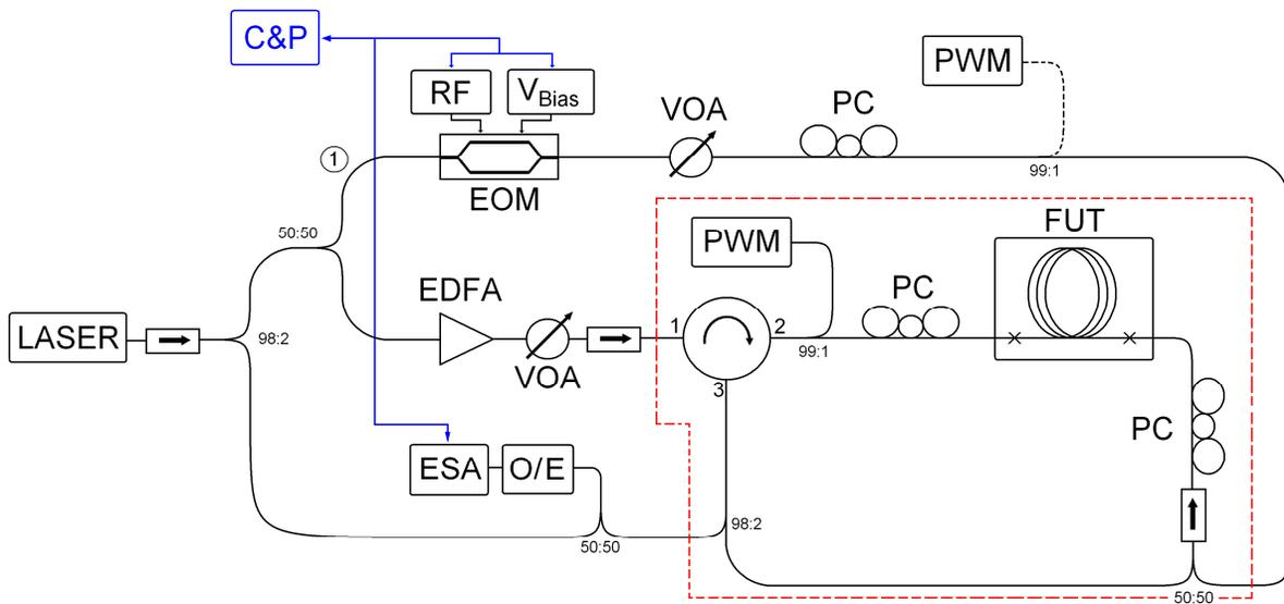
Figure 1. Experimental setup for Brillouin ring configuration. Setup composed by a variable optical attenuator (VOA), control and processing (C&P), optical to electrical converter (O/E), optical power meter (PWM) and polarization controller (PC).
