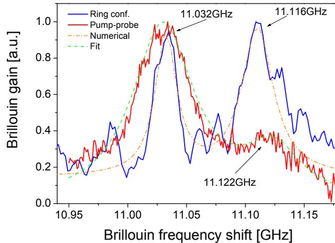
Figure 3. Brillouin spectra along the PCF shown in Figure 2 in the X-axis of polarization. The figure displays (Blue line) data from the ring cavity and (red line) data from the standard probe-pump configuration. It also shows the numerical (dotted-dashed line) Brillouin coupling coefficient and the fitting data.
