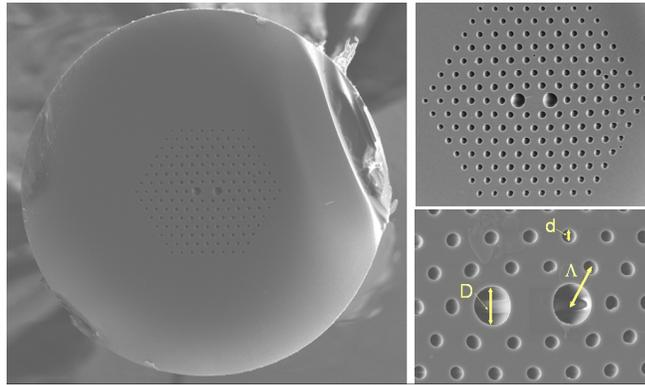
Figure 2. Polarization maintaining photonic crystal fiber.  $D=3\mu\text{m}$ ,  $d=1.7\mu\text{m}$  and  $\Lambda=3.75\mu\text{m}$ .
