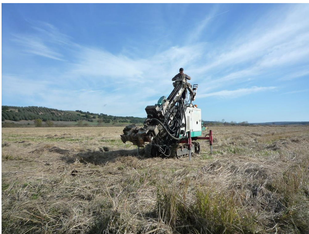
Figure 3.10 - Collection of the sediment core Laxique 1 in the Sado alluvial plain using a CASABRANCA M3D sampler.
