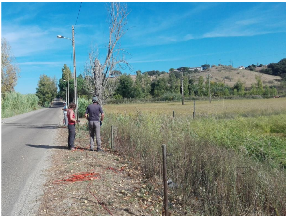
Figure 3.3 - Fieldwork for measurement of electrical resistivity tomography (ERT) in the Carrasqueira (Arez) tributary. The orange cable connects all the electrodes in the ground to perform the ERT profile. October 2017.
