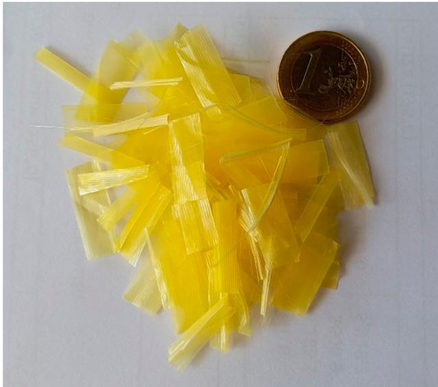
Figure 1. An illustration of polyolefin-aramid fibres.
