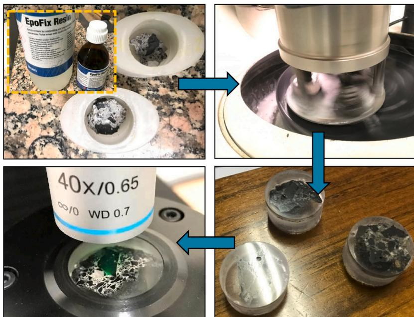
Fig. 5. Sample preparation and placement in the optical microscope.
