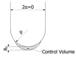
**Figure 1.** Control volume (area) for U-notch ( $2\alpha = 0$ ) under mode I loading.
