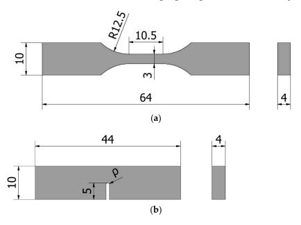
**Figure 4.** The geometry of the ABS AM specimens: (a) tensile specimens; (b) fracture specimens, with  $\rho$  varying from 0 mm up to 2 mm. Dimensions in mm.
