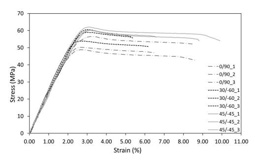
Figure 5. The stress-strain curves of the AM ABS material for the three different raster orientations.
