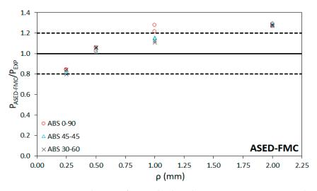
**Figure 9.** Comparison between fracture load predictions using ASED-FMC and experimental fracture loads.
