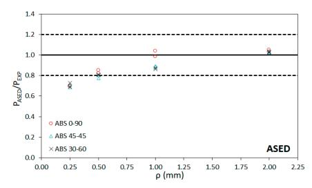
Figure 7. Comparison between fracture load predictions using ASED and experimental fracture loads.
