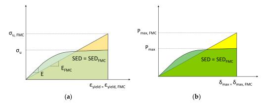
**Figure 3.** Real material and FMC material; (**a**) Tensile stress-strain curves; (**b**) Load-displacement curves of pre-cracked samples in fracture tests.
