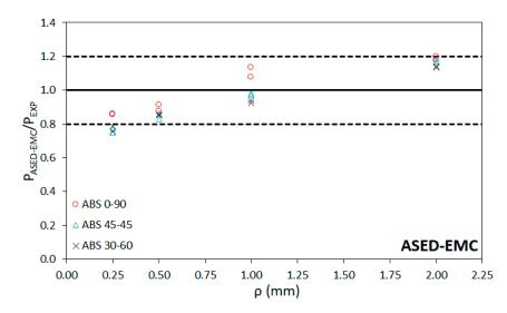
**Figure 8.** Comparison between fracture load predictions using ASED-EMC and experimental fracture loads.
