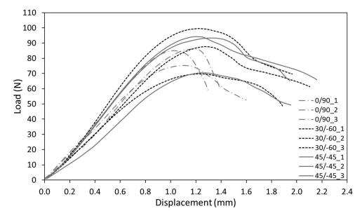
Figure 6. Load-displacement curves of the AM ABS for the three different raster orientations.
