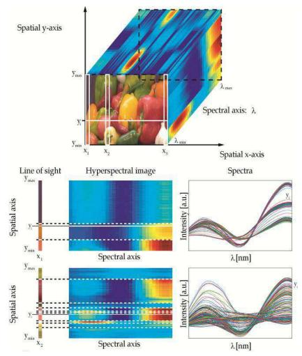
Fig. 1. HIS concept showing how the spectrum of a spatial point is recovered from an image
