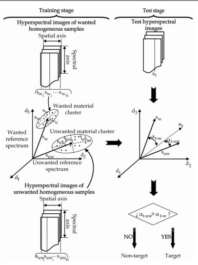
Fig. 8. SAM schematic description. "Training stage": calculation of the reference spectrum of each class ( $s_{uw}$  and  $s_w$ ). "Test stage" an unknown spectrum  $s_t$  is compared with these references for classification
