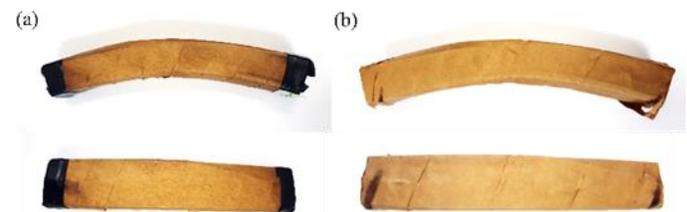
**Figure 9.** Results for  $d = 5$  mm in Ageing State I, for (a) the crepe paper in layer 4, (b) the Kraft paper in layer 2.
