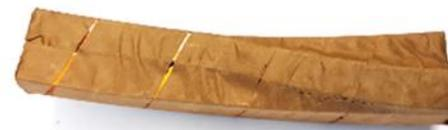
**Figure 10.** Results for  $d = 5$  mm in Ageing State I, for the Kraft paper in layer 1.
