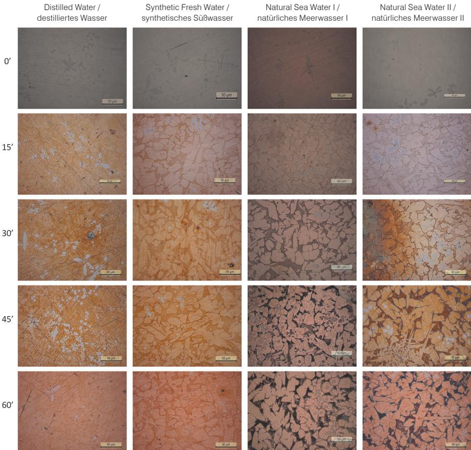
**Fig. 7:** Evolution of etching using US bath in different media.
