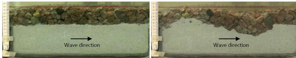
*Figure 1: Scour in front of rubble mound breakwaters.. Image from (Papadopoulos, 2013).*
