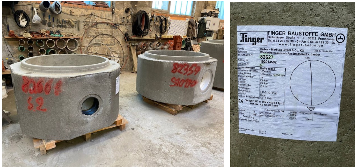
Figure 57: Manhole elements of the company Finger-Baustoffe GmbH with glued-on manhole information, right (Source: A. Juraboev, M. Bodenbender)
