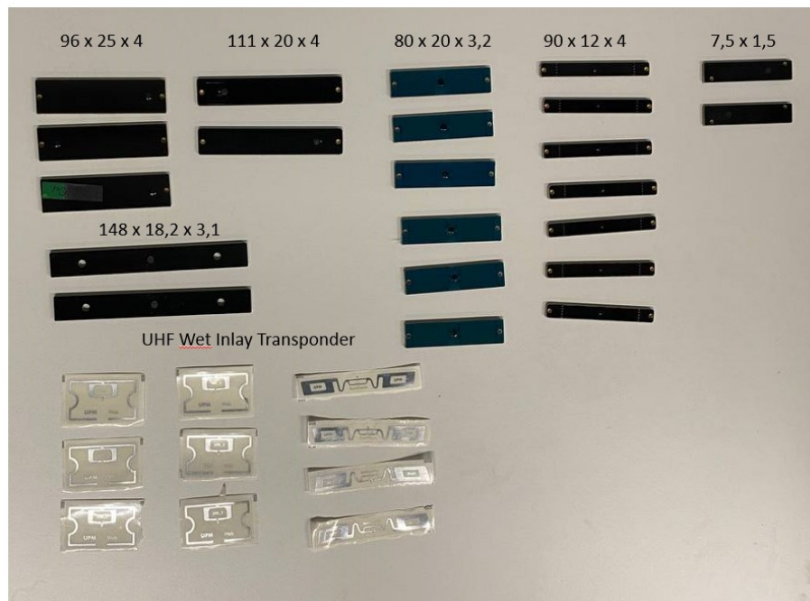
Figure 53: Tested UHF RFID tags with specification of dimensions (Source: A. Juraboev)
