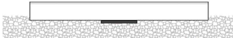
Figure 4: Types of RFID transponder insertion in building materials (modified) [25]
