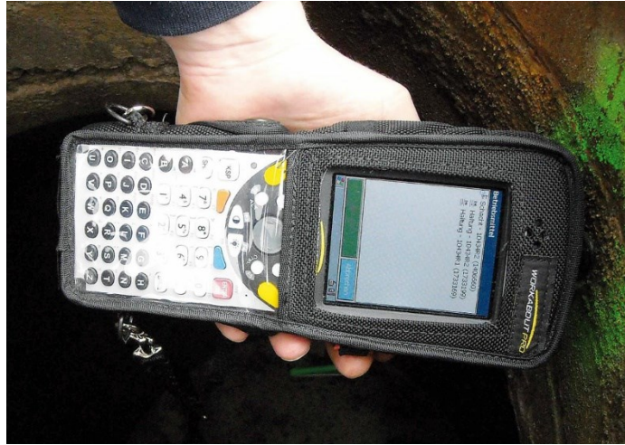
Figure 19: Identification of a Manhole using the Built-in RFID Transponder with the help of PDA Reader [82]
