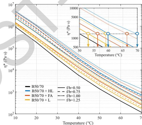
**Figure 5.** Results of the complex viscosity of the bitumen and asphalt mastics
