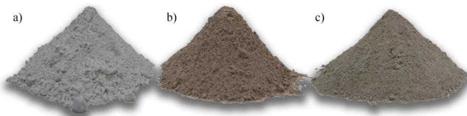
**Figure 1.** The fillers used sifted through an N°200 (0.08 mm) sieve. a) HL; b) FA; c) L
