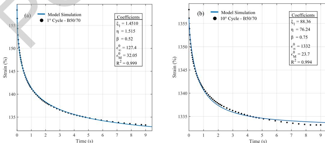
Figure 10. Rheological simulation of bitumen B50/70 for 3.2 kPa and 50°C. a) 1°cycle; b)10°cycle
