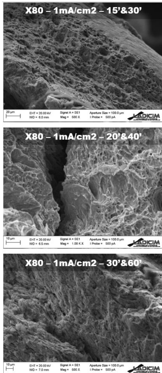
Figure 11 Fracture surfaces of X80 steel obtained by applying the SPT step loading technique when tested in a cathodic polarization environment of 1 mA/cm 2 ; images correspond to the sample tested under the final step protocol (the one that determines P_{th} ).
