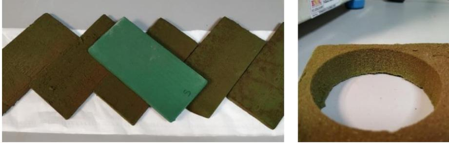
**Figure 13.** Results of the geofoam oxidation and alteration test.
