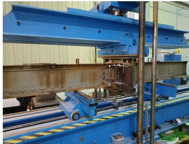
Figure 7. Laboratory test of the non-strengthened connection.
