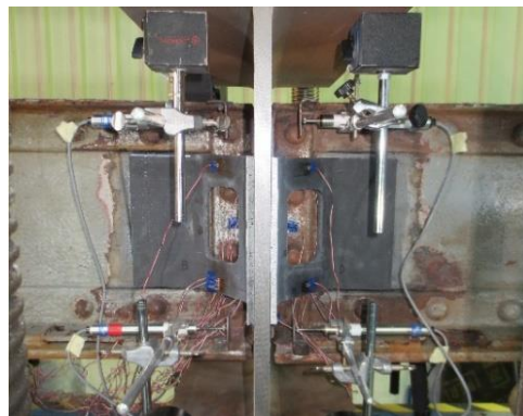
Figure 24. Test of the CFRP-strengthened connection.
