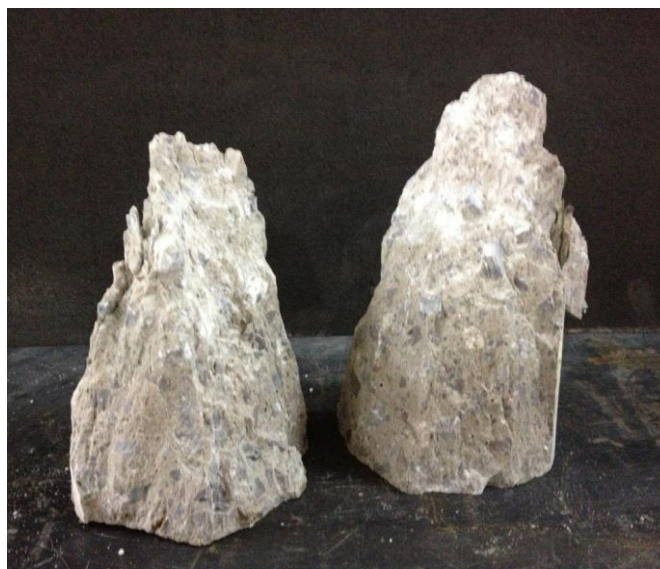
Figure 13. Comparison of the concrete fracture surface obtained at moderate (right) and high frequency (left).
