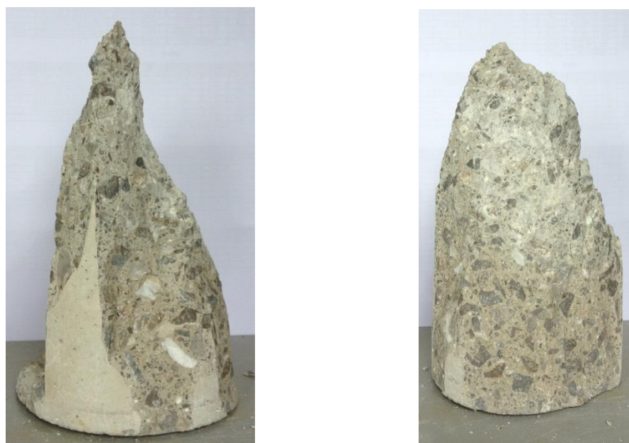
Figure 10. Fracture surface of a sample broken during a fatigue test, mode 2.
