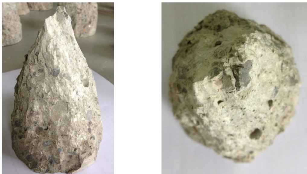
Figure 9. Fracture surface of a sample broken during a fatigue test, mode 1.
