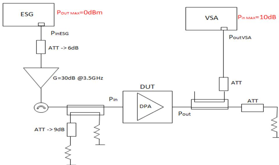
Fig. 45: Measure bench diagram.
