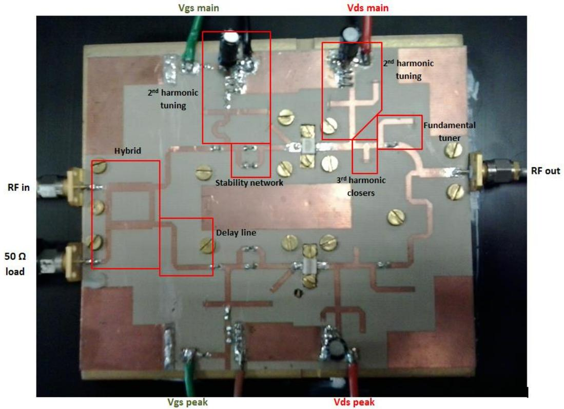
Fig. 43: Picture of the fabricated DPA with the most important parts highlighted.
