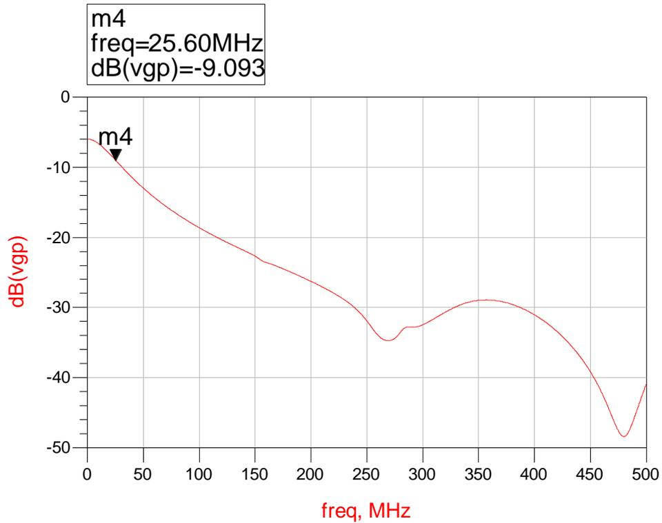
Fig. 29: Signal seen at the gate with a resistor in parallel.
