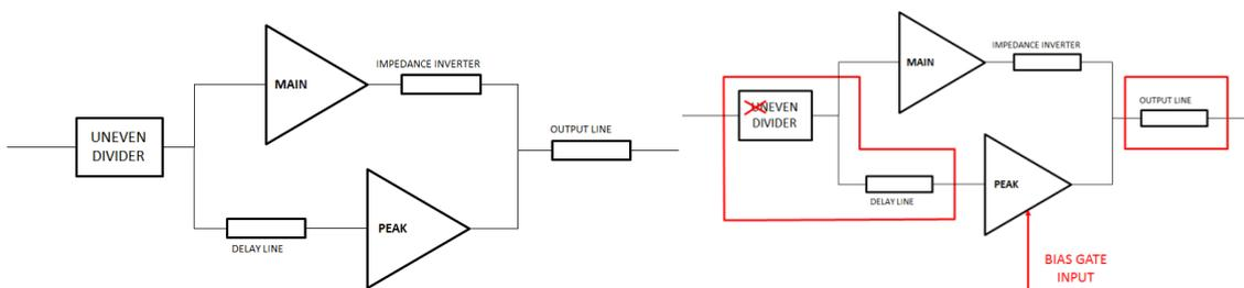
Fig. 1: Original design vs. changes proposed.
