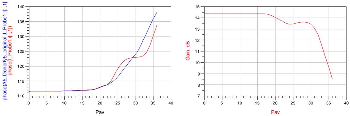
Fig. 10: Gain and phase with a threshold of 5 (the red ones). The blue one is the phase of the original design.
