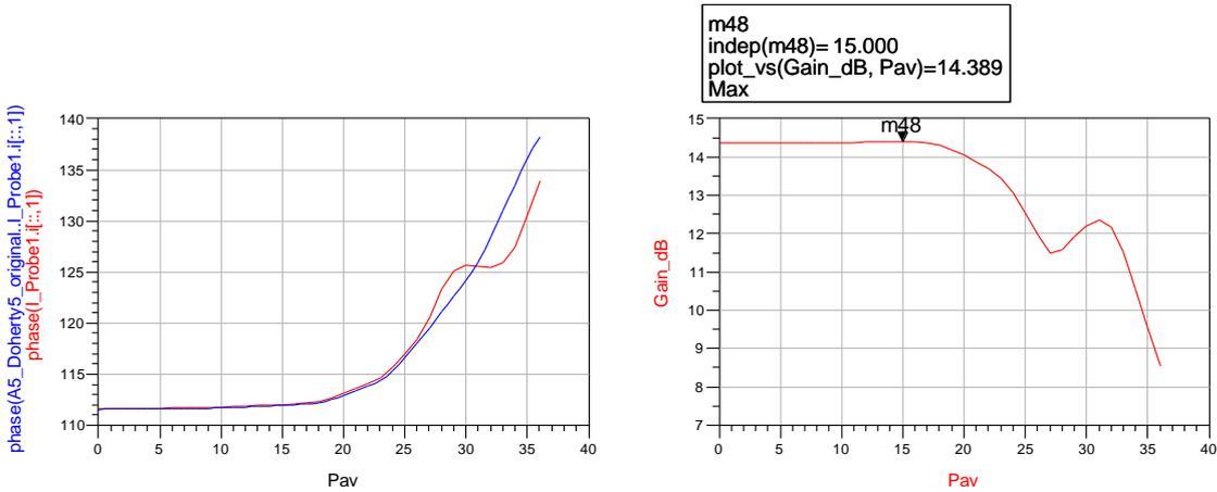
Fig. 24: Phase and gain with the threshold chosen.
