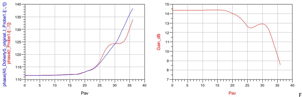
Fig. 8: Gain and phase with a threshold of 20 (the red ones). The blue one is the phase of the original design.
