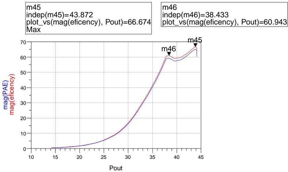
Fig. 25: Efficiency and PAE with the threshold chosen.
