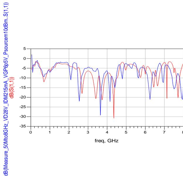
Fig. 50: S11 simulated (red) versus S11 measured (blue).
