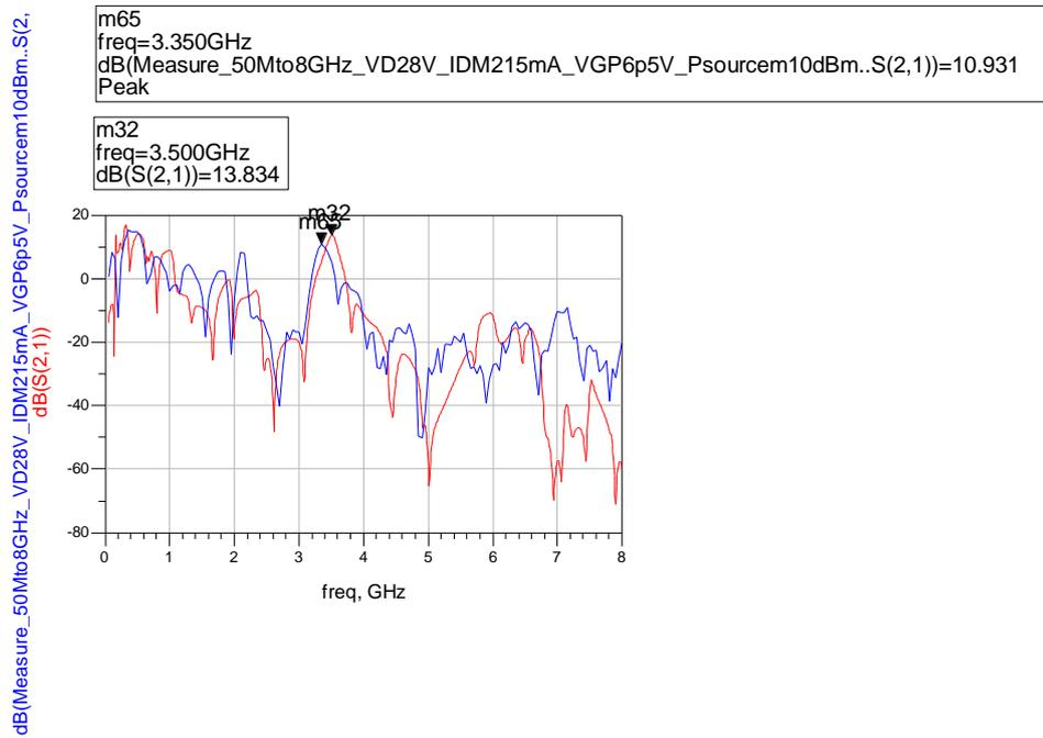
Fig. 49: S21 simulated (red) versus S21 measured (blue).
