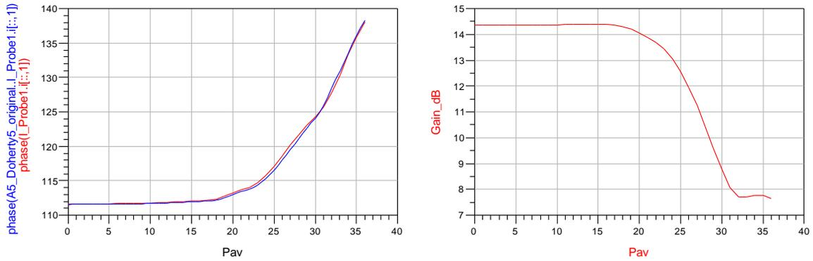
Fig. 6: Gain and phase with a threshold of 36 (the red ones). The blue one is the phase of the original design.
