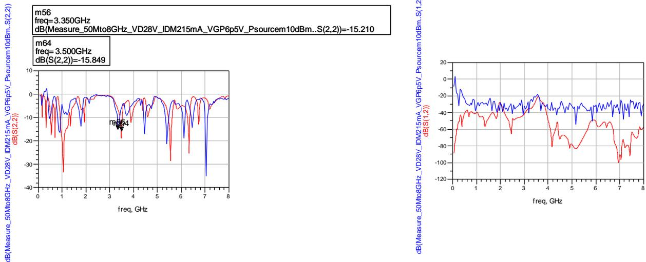
Fig. 51: S22 and S12 simulated (red) versus S22 and S12 measured (blue).
