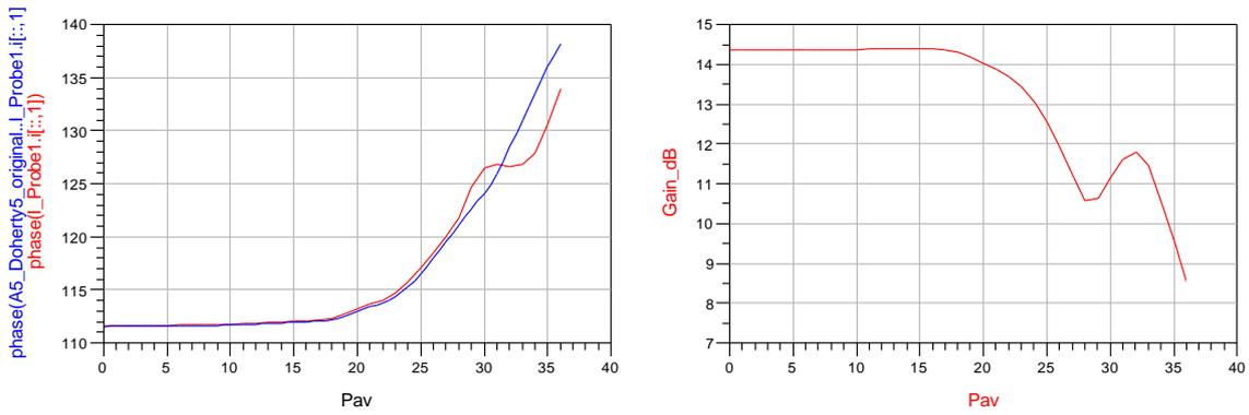
Fig. 7: Gain and phase with a threshold of 25 (the red ones). The blue one is the phase of the original design.
