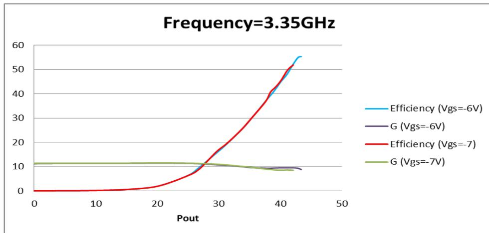
Fig. 48: Gain and efficiency with different peak's Vgs.
