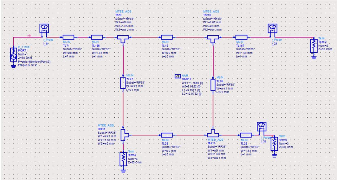
Fig. 4: Hybrid coupler design.
