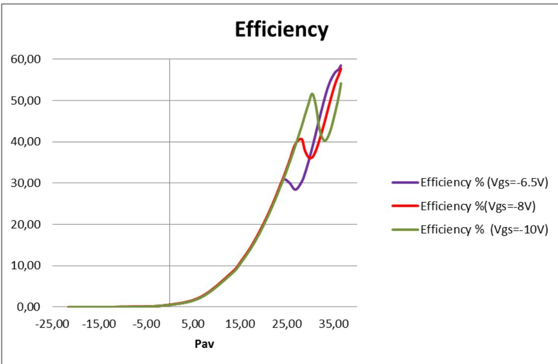
Fig. 59: Efficiency for the different Vgs.
