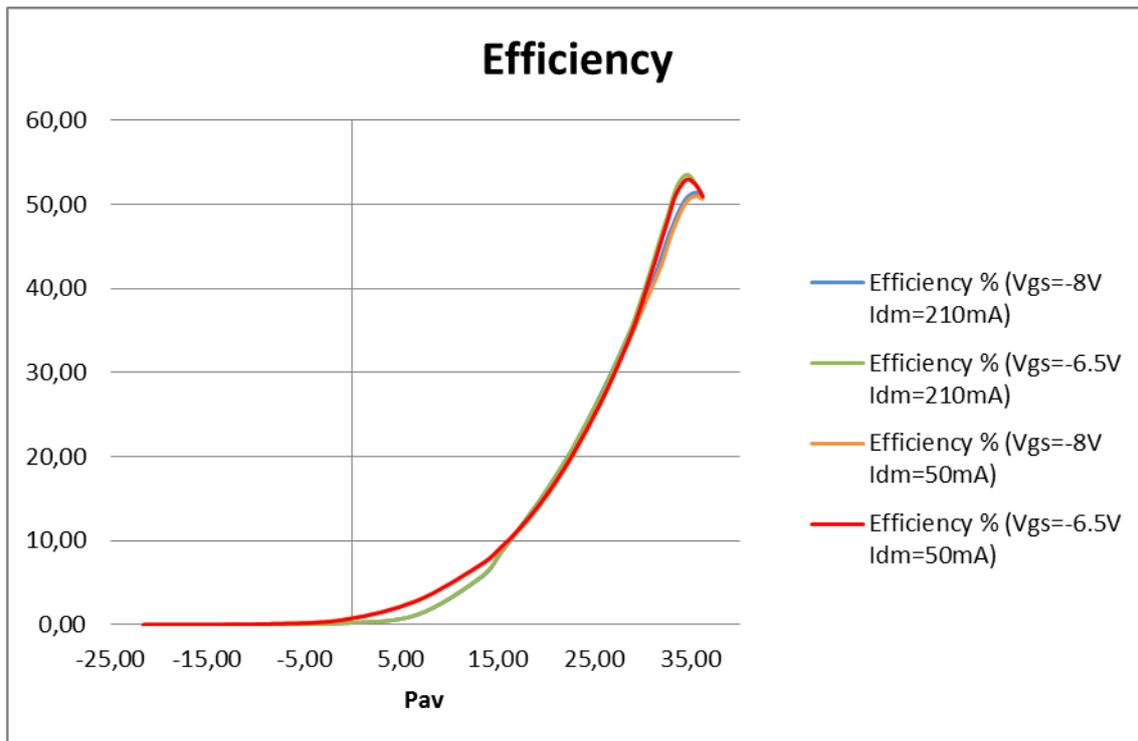
Fig. 62: Efficiency for the different bias.
