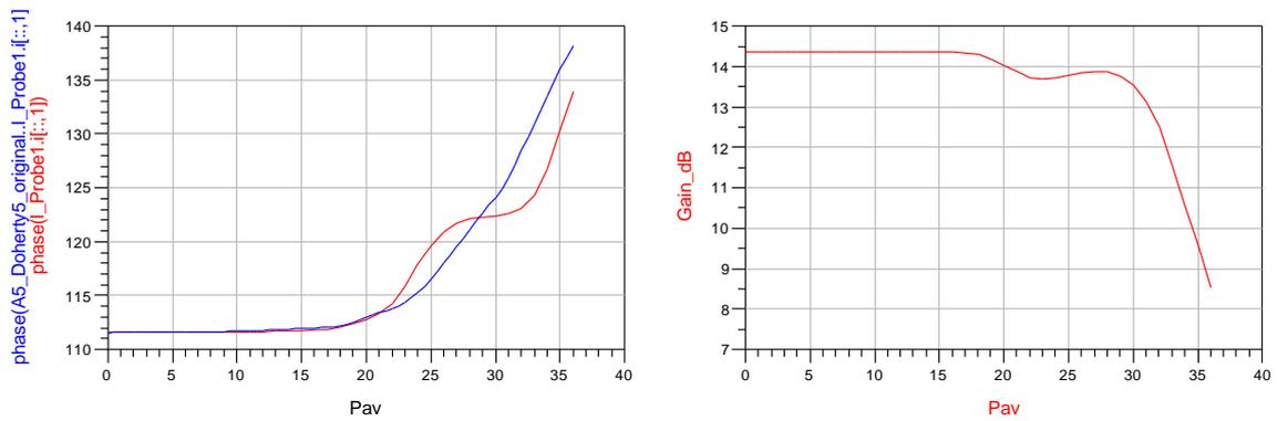
Fig. 11: Gain and phase with a threshold of 0 (the red ones). The blue one is the phase of the original design.
