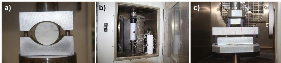
**Fig. 3.** Experimental set-up of (a) the tensile splitting tests, (b) uniaxial compression tests and (c) four-point bending tests.
