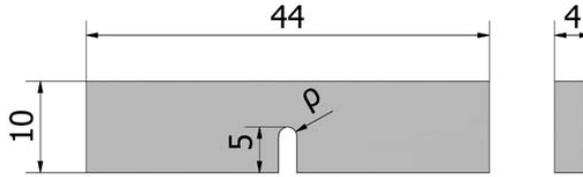
Fig. 3. Geometry of SENB fracture specimens. Dimensions in mm.
