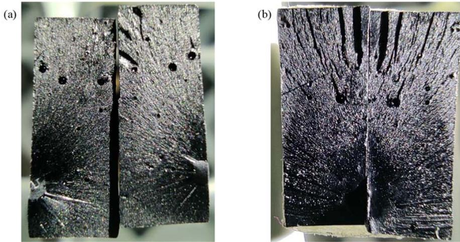
Fig. 7. Fracture surface of tensile specimens with different MWCNTs concentrations, revealing numerous internal defects: (a) 0.3 wt.% and (b) 0.5 wt.%.
