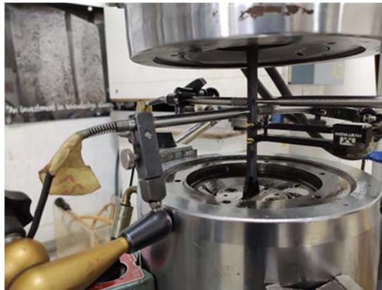
Fig. 2. Experimental set-up of tensile tests.
