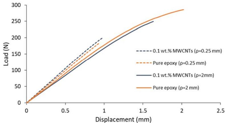
Fig. 5. Load-displacement curves of two different notch radii.
