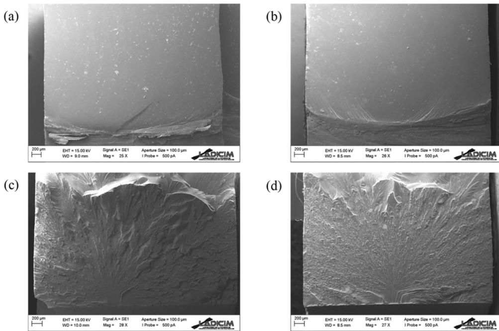
Fig. 8. SEM images obtained from fracture specimens; a) pure epoxy cracked specimen; b) 0.1 wt.% MWCNTs cracked specimen; c) pure epoxy notched (notch radius 2mm) specimen; d) 0.1 wt.% MWCNTs notched (notch radius 2mm) specimen.
