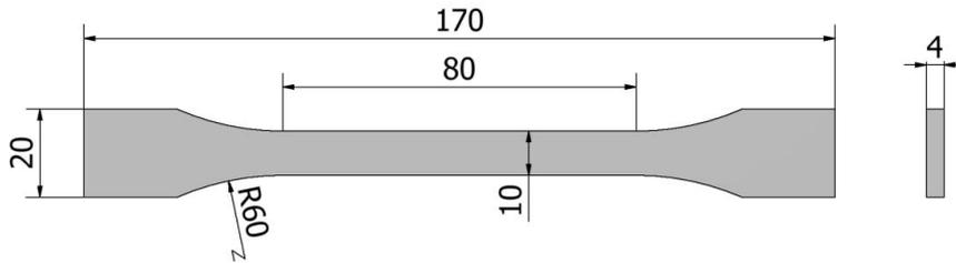
Fig. 1. Geometry of the tensile samples. Dimensions in mm.
