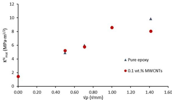
Fig. 6. Evolution of fracture toughness (average values) with notch radius for pure epoxy and by adding 0.1 wt.% of MWCNTs.
