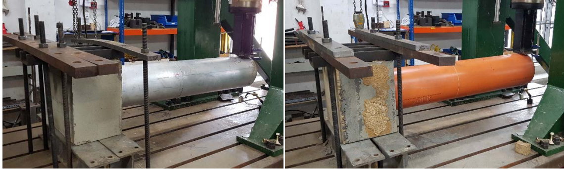
Figure 9. Experimental setup. Al6060-T66 (left); PVC (right).
