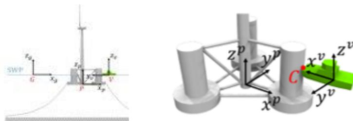
**Figure 4.** Contact between platform and CTV
