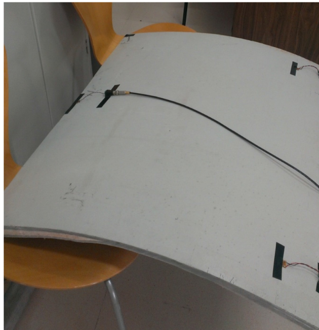
Fig. 16. Blade section with sensors for acoustic emission location Gomez Munoz and Garcia Marquez (2016).
