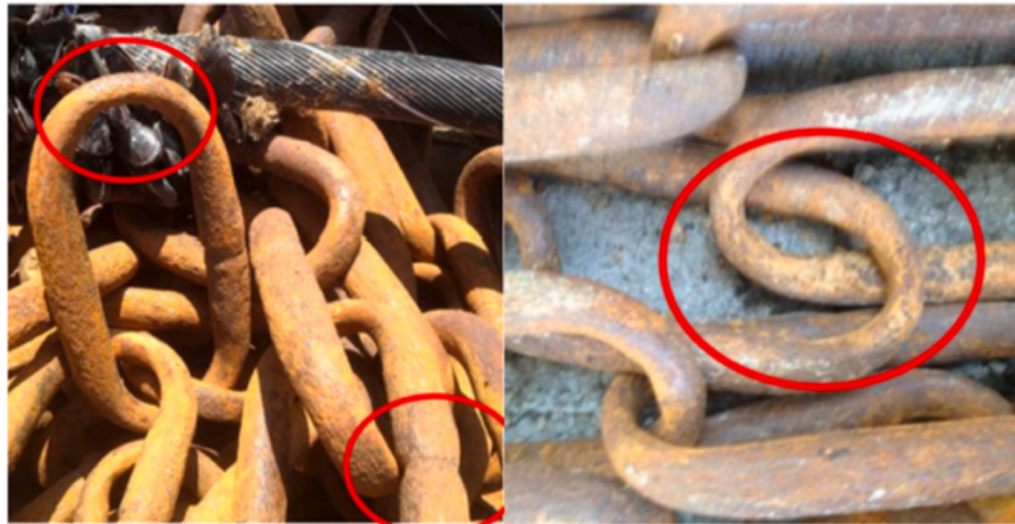
Fig. 8. Corrosion observed in catenary mooring lines for FOWT (Pham et al., 2019).
