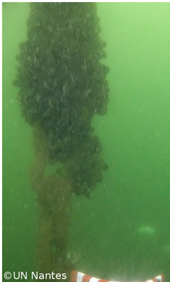
Fig. 10. Colonization of mussels on a mooring chain Decurey et al. (2020).
