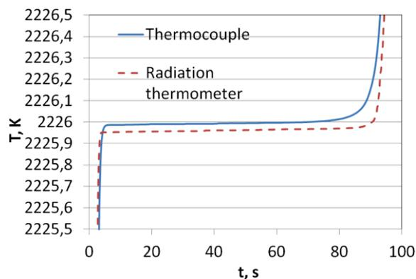
FIGURE 10. Melting plateau for Ru-C in the cell inside the furnace.
