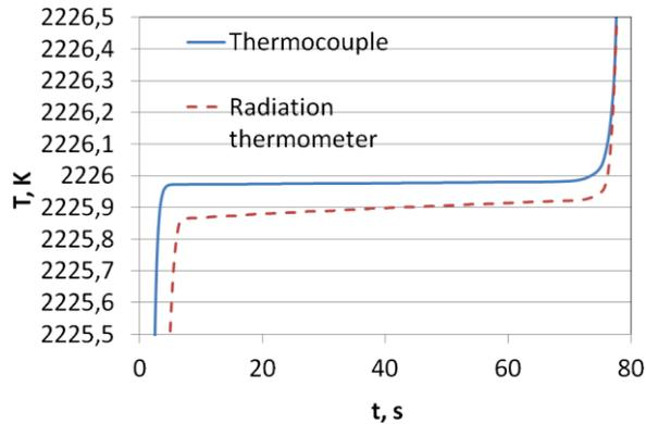
FIGURE 9. Melting plateau for Ru-C in the cell without furnace.
