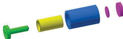
**FIGURE 3.** NPL HTFP design. Total length 40 mm. Internal cavity length 28.5 mm. Internal diameter 3 mm.
