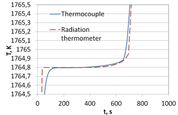
FIGURE 8. Melting plateau for Pd-C in the cell inside the furnace.
