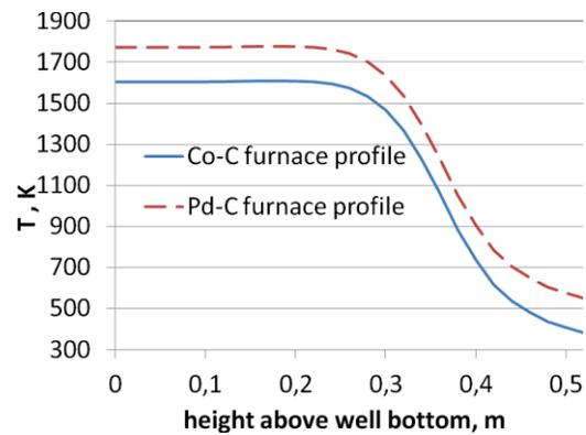
FIGURE 4. Furnace temperature profile for Co-C and Pd-C points.
