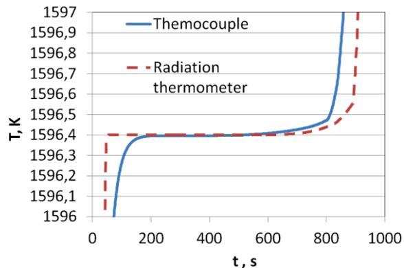
FIGURE 6. Melting plateau for Co-C in the cell inside the furnace.
