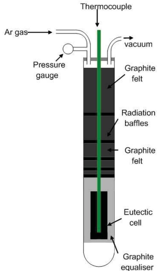
**FIGURE 2.** Schematic diagram of the cell holder and its assembly used for thermocouple calibrations.
