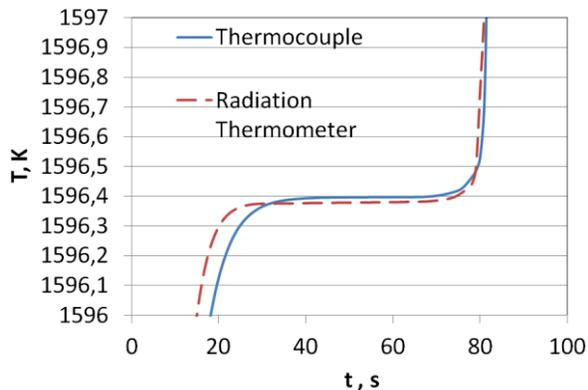
FIGURE 5. Melting plateau for Co-C in the cell without furnace.
