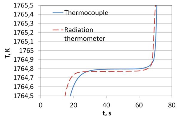
FIGURE 7. Melting plateau for Pd-C in the cell without furnace.
