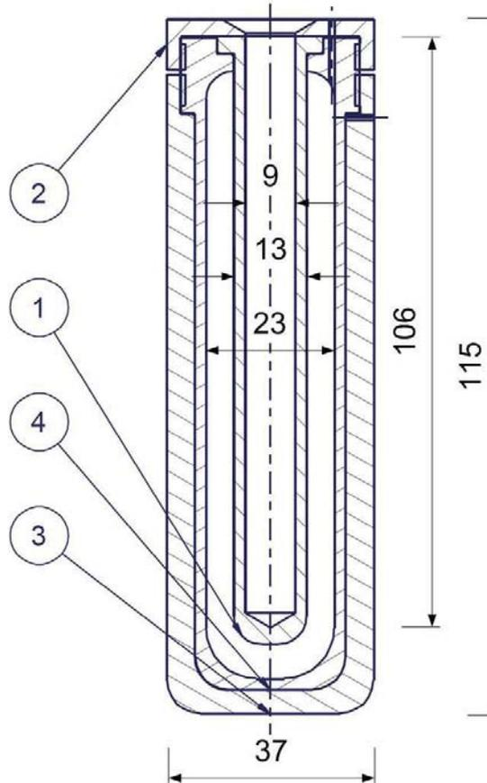
**FIGURE 1.** NPL HTFP cell design for thermocouple calibration. 1: thermowell, 2: top cap, 3: outer sleeve, 4: inner sleeve. Units in mm.
